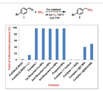
Fig. 2 Reductive amination of 4-bromobenzaldehyde: Activity of cobalt catalysts<sup>a</sup>. <sup>a</sup>Reaction conditions: 0.5 mmol 4-bromobenzaldehyde, 6 mol% Co-complex, (Co NPs), 5 bar NH $_3$ , 45 bar H $_2$ , 2.5 mL H $_2$ O-THF (1.5 : 1), 120 °C, 24 h, GC yields using n-hexadecane as standard.
