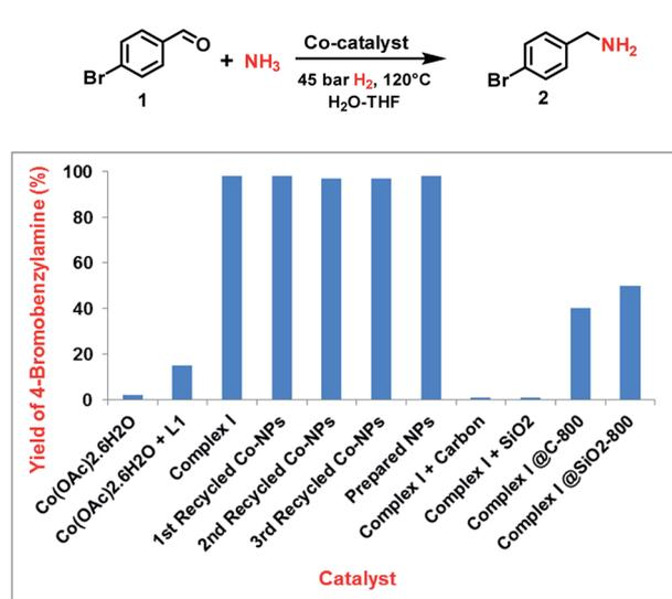
Fig. 2 Reductive amination of 4-bromobenzaldehyde: Activity of cobalt catalysts.<sup>a</sup> Reaction conditions: 0.5 mmol 4-bromobenzaldehyde, 6 mol% Co-complex, (Co NPs), 5 bar NH<sub>3</sub>, 45 bar H<sub>2</sub>, 2.5 mL H<sub>2</sub>O-THF (1.5 : 1), 120 °C, 24 h, GC yields using *n*-hexadecane as standard.
