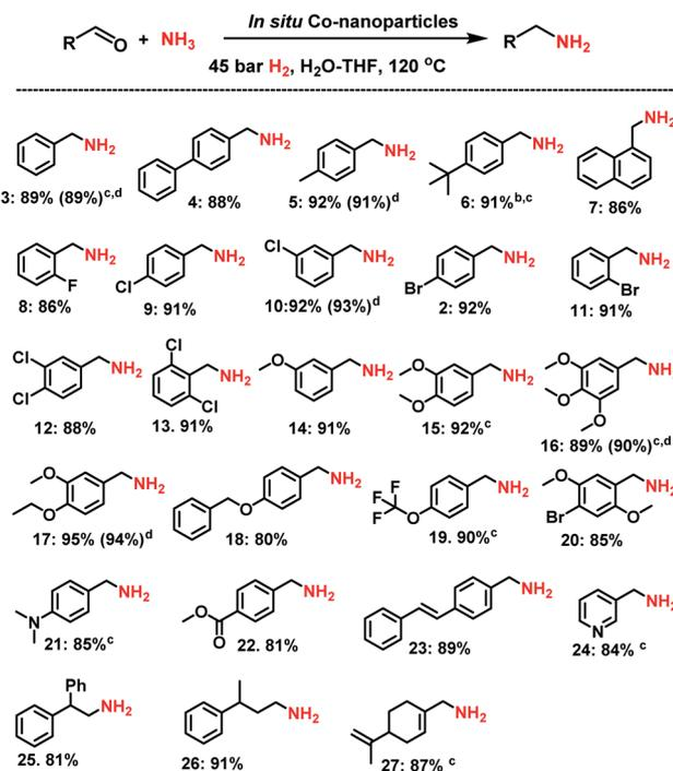
**Scheme 1** *In situ* generated Co-nanoparticles catalyzed synthesis of linear primary amines from aldehydes<sup>a</sup>. <sup>a</sup>Reaction conditions: 0.5 mmol aldehyde, 6 mol% complex I (22 mg), 5–7 bar NH<sub>3</sub>, 45 bar H<sub>2</sub>, 2.5 mL H<sub>2</sub>O–THF (1.5 : 1), 120 °C, 24 h, isolated yields. <sup>b</sup> Same as 'a' at 130 °C. <sup>c</sup> Same as 'a' in 2.5 mL H<sub>2</sub>O. <sup>d</sup> same as 'a' using prepared and isolated Co-NPs from complex I (2 mg; 6.5 mol% Co).
