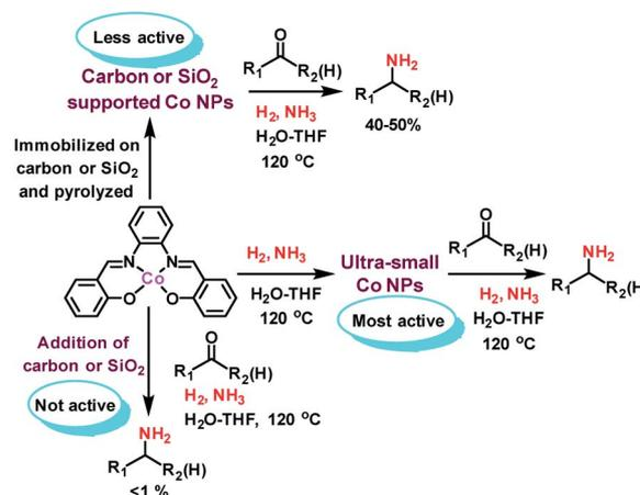
Fig. 3 Reductive amination of carbonyl compounds in presence of NH<sub>3</sub> and H<sub>2</sub> using different Co NPs produced from cobalt-salen complex.
