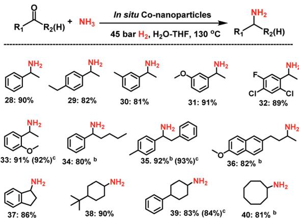
**Scheme 2** Synthesis of branched primary amines from ketones using *in situ* generated Co-nanoparticles<sup>a</sup>. <sup>a</sup>Reaction conditions: 0.5 mmol ketone, 6 mol% complex I (22 mg) 5–7 bar NH<sub>3</sub>, 45 bar H<sub>2</sub>, 2.5 mL H<sub>2</sub>O, 130 °C, 24 h, isolated yields. <sup>b</sup> Same as 'a' in H<sub>2</sub>O–THF (1.5 : 1 ratio). <sup>c</sup>Using prepared and isolated Co-NPs from complex I (2 mg; 6.5 mol% Co).
