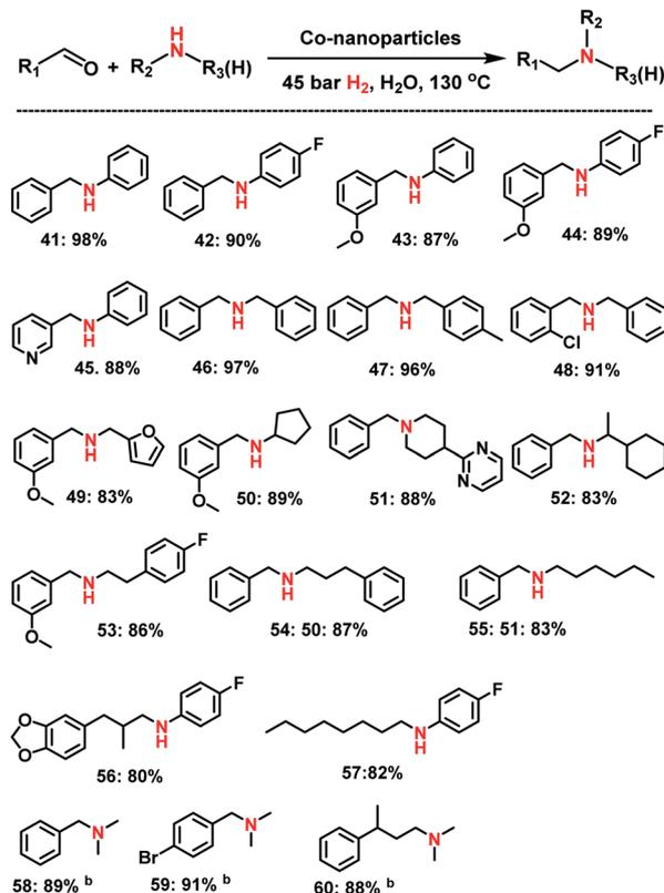
**Scheme 3** Synthesis of secondary, tertiary and *N*-methyl amines using Co-nanoparticles prepared from complex I<sup>a</sup>. <sup>a</sup>Reaction conditions: 0.6 mmol aldehyde, 0.5 mmol amine, 2 mg Co-NPS (6.5 mol% Co), 45 bar H<sub>2</sub>, 2.5 mL H<sub>2</sub>O, 130 °C, 20 h, isolated yields. <sup>b</sup>Same as 'a' using 1 mL aq. *N,N'*-dimethylamine instead of amine.
