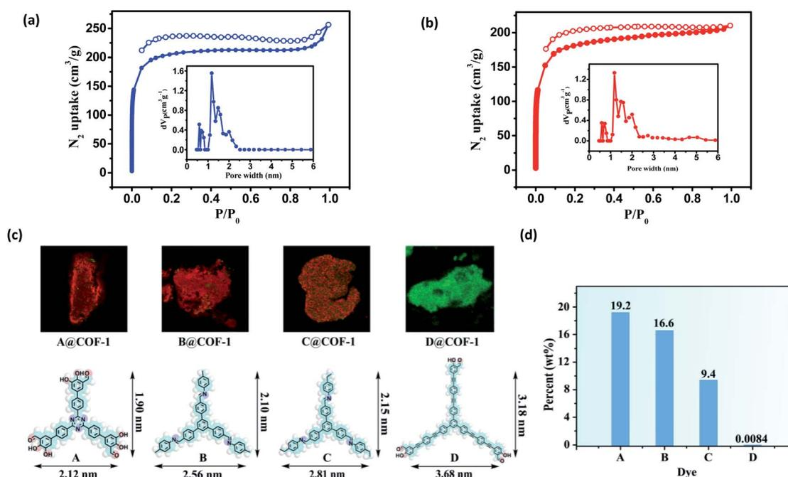
Fig. 4 (a)  $\text{N}_2$  adsorption–desorption isotherms (77 K) and pore size distribution profiles of COF-1; (b)  $\text{N}_2$  adsorption–desorption isotherms (77 K) and pore size distribution profiles of COF-2. (c) CFM images obtained from COF-1 after incubation with dyes A–D, respectively. (d) Different dye uptake released from COF-1 by UV-vis spectroscopy.
