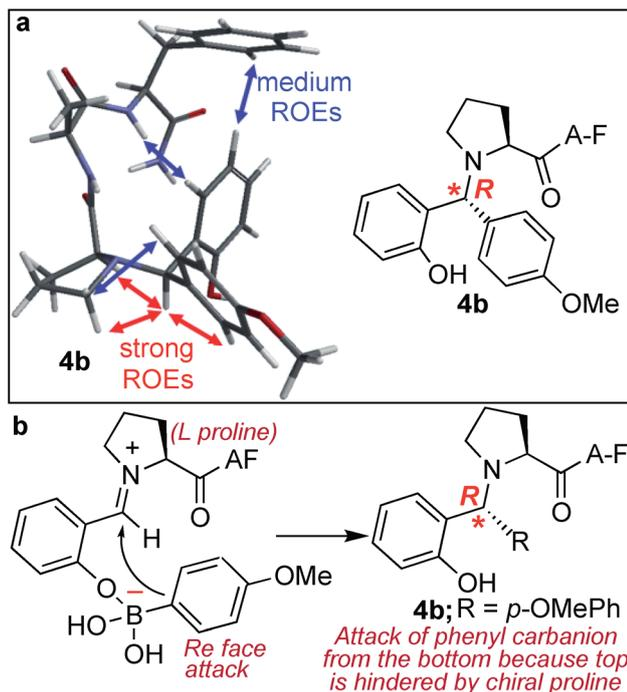
Fig. 5 Chemo- and stereo-selective SASP bioconjugation under physiological conditions. (a) NMR ROEs of Petasis product **4b** are consistent with *R* configuration from molecular mechanics Monte Carlo. (b) Plausible pathway for high stereoselectivity.
