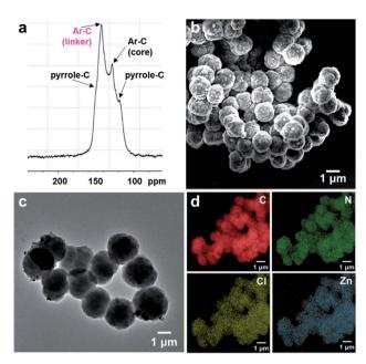
Fig. 2 (a) <sup>13</sup>C solid-state NMR spectrum of PV-COF with peaks assigned to relevant carbon atoms; (b) SEM image of PV-COF shows spherical particles with an average size of 1.4 μm; (c) TEM image of PV-COF; (d) elemental mapping of Zn-PV-COF showing an even distribution of constituent elements (C, N, Cl and Zn).
