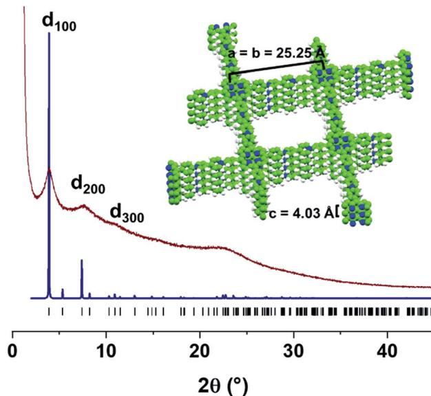
Fig. 3 Experimental PXRD pattern of the as-synthesized PV-COF (brown line) compared with the simulated pattern using the optimized crystal model (blue line), built in the  $P4$  unit cell with  $a = b = 25.25 \text{ \AA}$ , and  $c = 4.03 \text{ \AA}$ . Inset: space-filling view of stacked layers along  $x$  and  $y$  axes.
