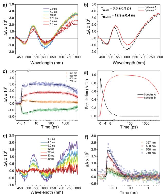
Fig. 8 Femtosecond transient absorption spectra (fsTA) of (a) Ant910Me<sub>2</sub>-CB[8]<sub>2</sub> complexes in D<sub>2</sub>O at 298 K following a laser pulse of 414 nm (1 μJ per pulse). Fitting from the raw data using a kinetic model A → B → GS gives (b) species associated spectra, (c) wavelength fitting, and (d) model population kinetics. (e) Nanosecond transient absorption spectra (nsTA) of species B and (f) its kinetic fitting at selected wavelength using mono-exponential model.
