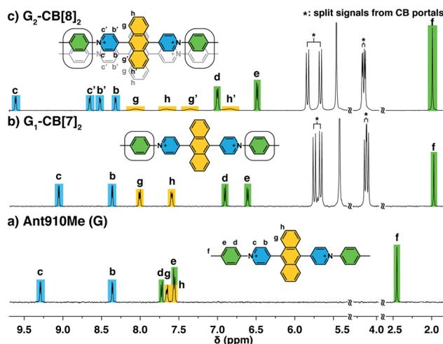
Fig. 2  $^1\text{H}$  NMR spectra (500 MHz) of (a) **Ant910Me** (G), and (b) its complexation with 2 equiv. of CB[7] ( $G_1\text{-CB}[7]_2$ ), or (c) with 1 equiv. of CB[8] ( $G_2\text{-CB}[8]_2$ ) in  $\text{D}_2\text{O}$  with a uniform guest concentration of 100  $\mu\text{M}$  at 298 K. The  $\text{Cl}^-$  counterions are omitted for clarity.
