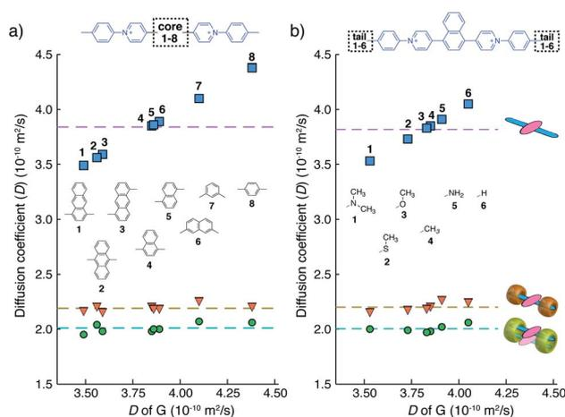
Fig. 3 Diffusion coefficients obtained from DOSY NMR for G (rectangles),  $G_1\text{-CB}[7]_2$  (triangles), and  $G_2\text{-CB}[8]_2$  (circles) with variation in (a) fluorophore cores or (b) substituted tails. ( $\text{D}_2\text{O}$  solution with a uniform guest concentration of 100  $\mu\text{M}$  at 298 K.) The  $\text{Cl}^-$  counterions are omitted for clarity.
