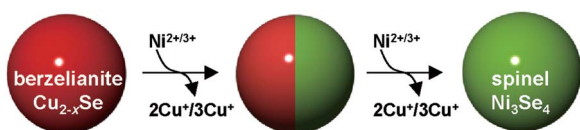
Scheme 1 Schematic of the cation exchange reaction of \text{ber-Cu}_{2-x}\text{Se} NCs with Ni cations.
