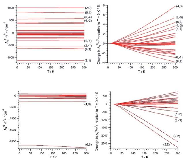
Fig. 2 Absolute (left) and relative to  $T = 0$  K (right) thermal evolution of the CFPs of  $[\text{U}(\text{Cp}^{\text{ttt}})_2]^+$  (top) and  $\text{UTp}_3$  (bottom). Some CFPs are identified as  $(k, q)$ , where  $k$  and  $q$  are the scripts  $k = 2, 4, 6$  and  $q = -k, \dots, +k$ .
