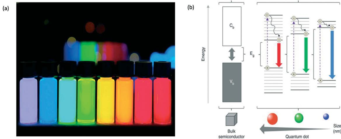
Fig. 1 (a) The different colours that QDs give rise to according to the energy emitted by the crystal; (b) the colour and size of the QD based on the energy level properties.<sup>3,16</sup>
