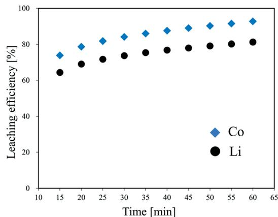
Fig. 4 Effect of time on the leaching efficiency of Li and Co during the continuous hydrothermal leaching of LiCoO<sub>2</sub> with H<sub>3</sub>Cit.
