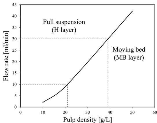
Fig. 2 Flow pattern map of the  $\text{LiCoO}_2$  slurry.
