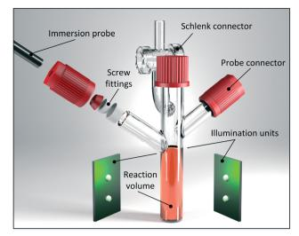
Fig. 2 Representation of the developed setup for studying photocatalytic reaction kinetics. The setup allows simultaneous LED irradiation and in situ monitoring by various PAT techniques.
