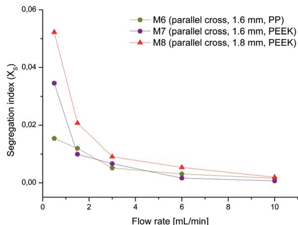
Fig. 8 Segregation index of PEEK mixers (M7, M8) and PP mixer M6.
