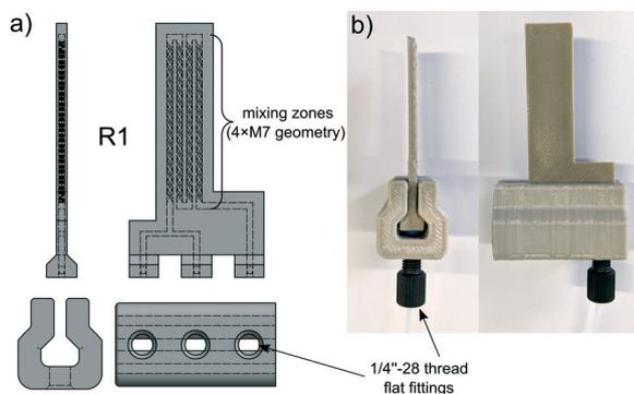
Fig. 2 CAD drawing (a) and photograph (b) with a connected 1/4"-28 fitting of reactor R1.
