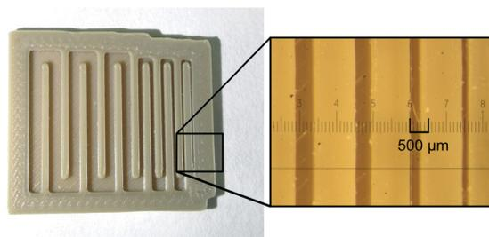
Fig. 9 Test piece for channel width measurements.
