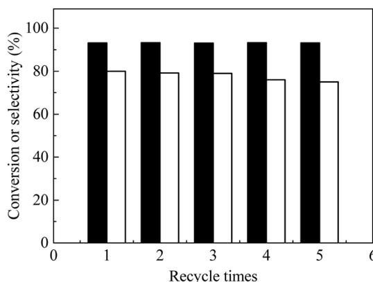
**Fig. 7** Recycle of catalyst to obtain ethyl levulinate (EL) direct from furfural alcohol (FAL) with bifunctional nanofiber catalyst. Reaction conditions: 0.1 g FAL, 0.09 g catalyst, 3 mL ethanol, reaction temperature, 150 °C, reaction time, 6 h. Black bars: FAL conversion, white bars: EL selectivity.
