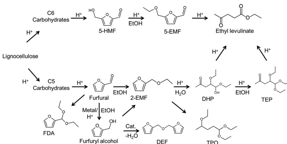
**Scheme 1** Probable reaction pathway for the conversion of carbohydrates in ethanol over acid catalyst 5-hydroxymethylfurfural (5-HMF), 5-ethoxymethylfurfural (5-EMF), 2-(ethoxymethyl)furan (2-EMF), 2,2'-difurfuryl ether (DEF), furfural diethyl acetal (FDA), 4,5,5-triethoxypentan-2-one (TEP), 4,5-diethoxy-5-hydroxypentan-2-one (DHP) and 2,5,5-triethoxypentan-2-one (TPO).
