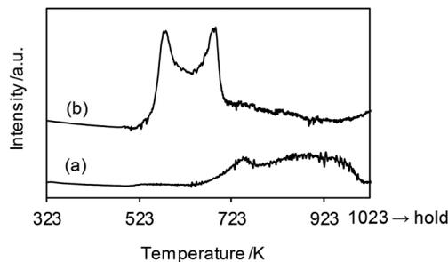
**Fig. 6** H<sub>2</sub>-TPR profiles of (a) WO<sub>3</sub>-ZrO<sub>2</sub> (WO<sub>3</sub> = 10 wt%) and (b) ReO<sub>x</sub>/WO<sub>3</sub>-ZrO<sub>2</sub> (Re = 1 wt%, WO<sub>3</sub> = 10 wt%). Measurement conditions: sample weight 50 mg, H<sub>2</sub>/Ar = 5/95, 10 K min<sup>-1</sup>. The H<sub>2</sub> consumption amount is summarized in Table 4.
