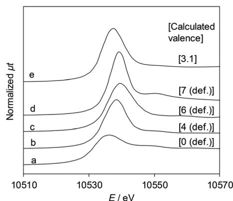
**Fig. 5** Re  $L_3$ -edge XANES spectra and the Re valence calculated using the white line area. (a) Re powder, (b)  $\text{ReO}_2$ , (c)  $\text{ReO}_3$ , (d)  $\text{Re}_2\text{O}_7$ , and (e)  $\text{ReO}_x/\text{WO}_3\text{-ZrO}_2$  after the reaction (reaction conditions: 2,5-DHF 0.15 g, water 0.03 g, catalyst 0.15 g, 1,4-dioxane 4 g,  $\text{H}_2$  8 MPa, 413 K, 4 h). The relationship between the white line area and Re valence is shown in Table S4 and Fig. S4, ESI<sup>†</sup>
