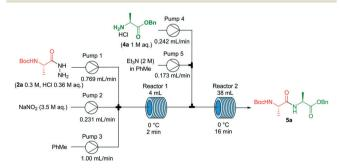
**Scheme 2** Continuous-flow setup for the acyl azide formation and subsequent amide coupling for *N*-Boc-L-Ala-NHNH<sub>2</sub> as substrate and amide coupling partner.
