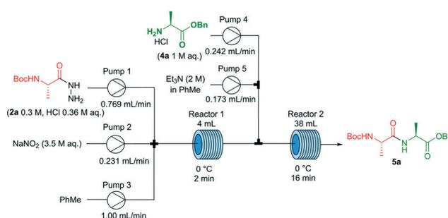
**Scheme 2** Continuous-flow setup for the acyl azide formation and subsequent amide coupling for *N*-Boc-*L*-Ala-NHNH<sub>2</sub> as substrate and amide coupling partner.
