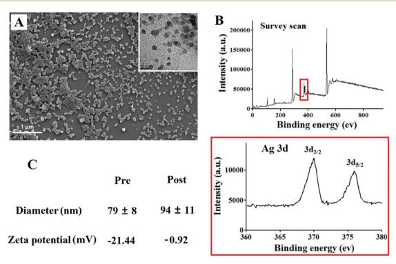
Fig. 1 (A) SEM image of PEGylated SLS NPs; inset: high-resolution TEM image highlighting the anchored Ag NPs. (B) XPS result of the SLS NPs and silver element. (C) DLS and zeta-potential profiles of the SLS NPs pre- and post-PEGylation.
