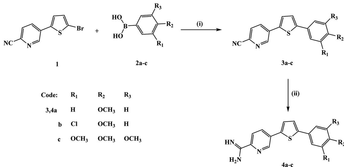
**Fig. 1** Synthesis scheme for the new thienylpicolinamide derivatives. Reagents and conditions: (i) Pd(PPh<sub>3</sub>)<sub>4</sub>, anhydrous K<sub>2</sub>CO<sub>3</sub>, 1,4-dioxane; (ii) (a) LiN(TMS)<sub>2</sub>, (b) ethanol/HCl (gas).
