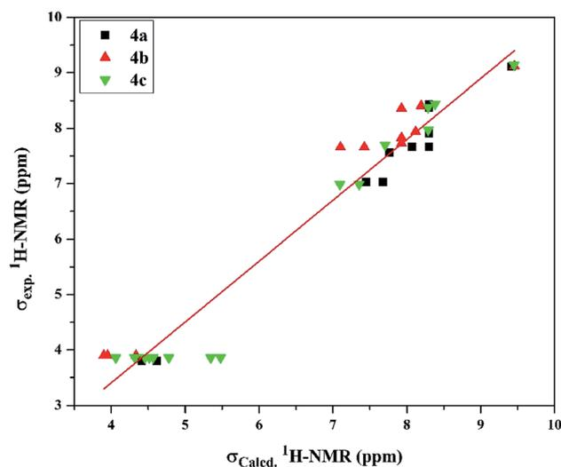
Fig. 3 The linear regression between experimental and DFT calculated <sup>1</sup>H NMR chemical shifts of the investigated cationic picolinamidines **4a-c**.
