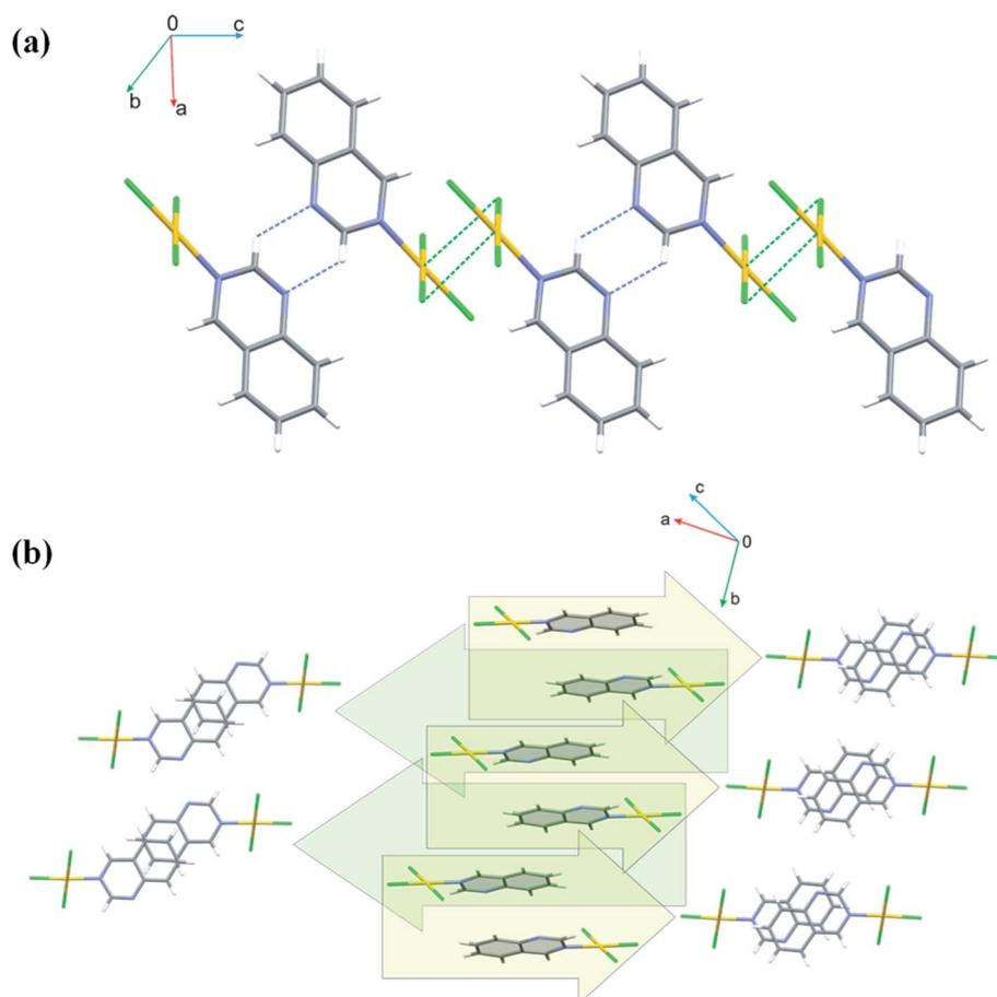
Fig. 3 Packing of the molecules of **1**. The figure illustrates pairs of the centrosymmetric dimers formed *via* C–H $\cdots$ N hydrogen bonds and Au $\cdots$ Cl interactions (a); columnar  $\pi\cdots\pi$  stacking, and two different modes of molecular overlap within the column (b).
