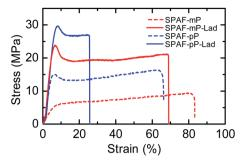
Fig. 5 Stress–strain curves of SPAF-P and SPAF-P-Lad membranes at 80  $^{\circ}$ C and 60% RH.
