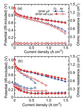
**Fig. 6** IR-included polarization curves and ohmic resistances of SPAF-pP (1.85 meq.  $g^{-1}$ , 27  $\mu$ m) and SPAF-mP-Lad (2.01 meq.  $g^{-1}$ , 26  $\mu$ m) membranes at 80 °C, (a) 100% RH and (b) 30% RH.
