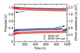
Fig. 7  $\,$  OCV hold test of SPAF- $p{\rm P}$  and SPAF- $m{\rm P-Lad}$  cells at 80  $^{\circ}{\rm C}$  and 30% RH with  ${\rm H_2}$  and air.
