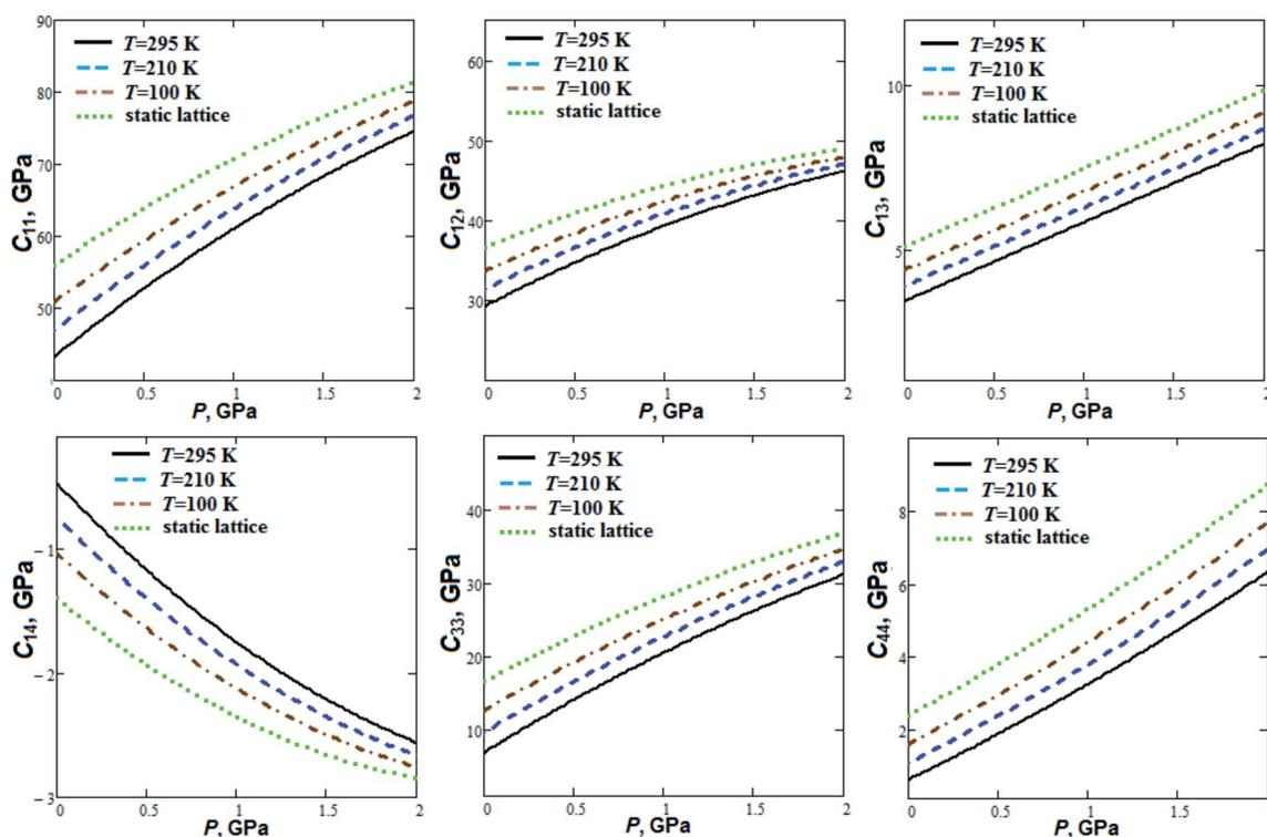
**Fig. 2** Calculated independent elastic constants as semi-empirical functions of pressure for guanidinium perchlorate at  $T = 295$  K (solid lines), 210 K (dashed lines), 100 K (dash-dotted lines) and at static lattice (dotted lines).  $C_{11} = 43.3$ ,  $C_{12} = 29.3$ ,  $C_{13} = 3.4$ ,  $C_{14} = -0.5$ ,  $C_{33} = 6.9$ ,  $C_{44} = 0.6$  GPa (at  $T = 295$  K).
