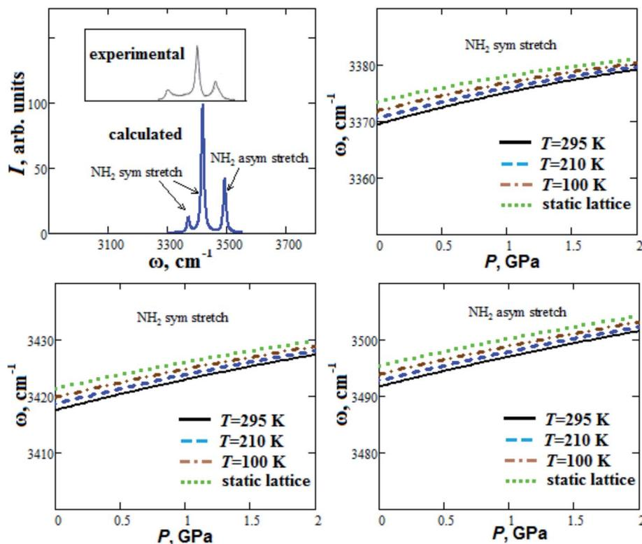
Fig. 5 Calculated Raman spectrum and semi-empirical pressure dependencies of frequencies  $\omega$  of  $\text{NH}_2$  stretch modes for guanidinium perchlorate at  $T = 295$  K (solid lines), 210 K (dashed lines), 100 K (dash-dotted lines) and at static lattice (dotted lines). Experimental Raman spectrum corresponds to ambient conditions.<sup>21</sup>
