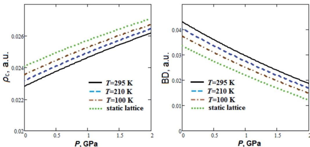
Fig. 4 Calculated semi-empirical pressure dependencies of electron density at bond critical points ( $\rho_c$ ) and bond degree (BD) for hydrogen bonds in guanidinium perchlorate at  $T = 295$  K (solid lines), 210 K (dashed lines), 100 K (dash-dotted lines) and at static lattice (dotted lines).
