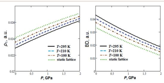
Fig. 4 Calculated semi-empirical pressure dependencies of electron density at bond critical points ( $\rho_c$ ) and bond degree (BD) for hydrogen bonds in guanidinium perchlorate at T=295 K (solid lines), 210 K (dashed lines), 100 K (dash-dotted lines) and at static lattice (dotted lines).
