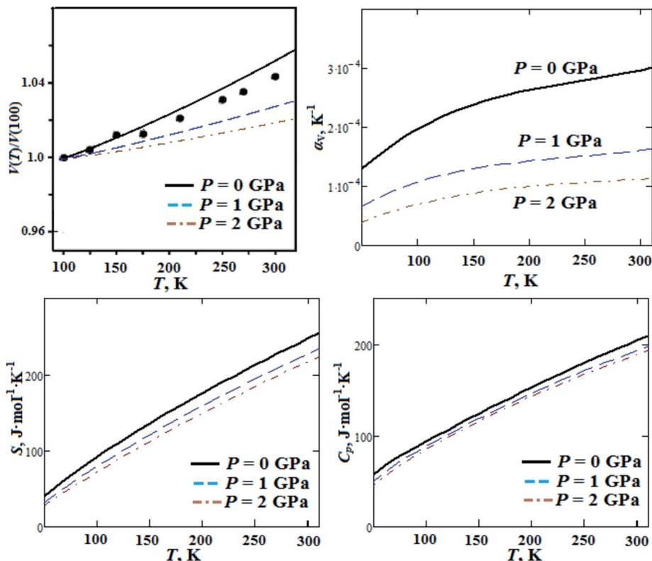
Fig. 6 Calculated temperature dependencies of relative volume, volume thermal expansion coefficient, entropy  $S$  and heat capacity  $C_p$  for guanidinium perchlorate at ambient pressure (solid lines),  $P = 1$  GPa (dashed lines) and  $P = 2$  GPa (dash-dotted lines). Experimental points correspond to ambient pressure.<sup>18</sup>
