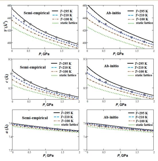
Fig. 1 Calculated semi-empirical and *ab initio* pressure dependencies of lattice parameters and volume for guanidinium perchlorate at T = 295 K (solid lines), 210 K (dashed lines), 100 K (dash-dotted lines) and at static lattice (dotted lines). Experimental points correspond to T = 295 K.<sup>22</sup>
