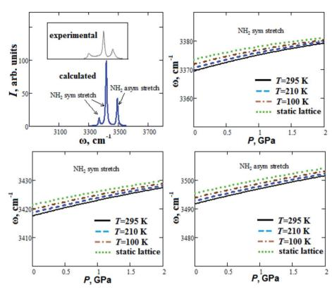
Fig. 5 Calculated Raman spectrum and semi-empirical pressure dependencies of frequencies  $\omega$  of NH<sub>2</sub> stretch modes for guanidinium perchlorate at T=295 K (solid lines), 210 K (dashed lines), 100 K (dash-dotted lines) and at static lattice (dotted lines). Experimental Raman spectrum corresponds to ambient conditions.<sup>21</sup>
