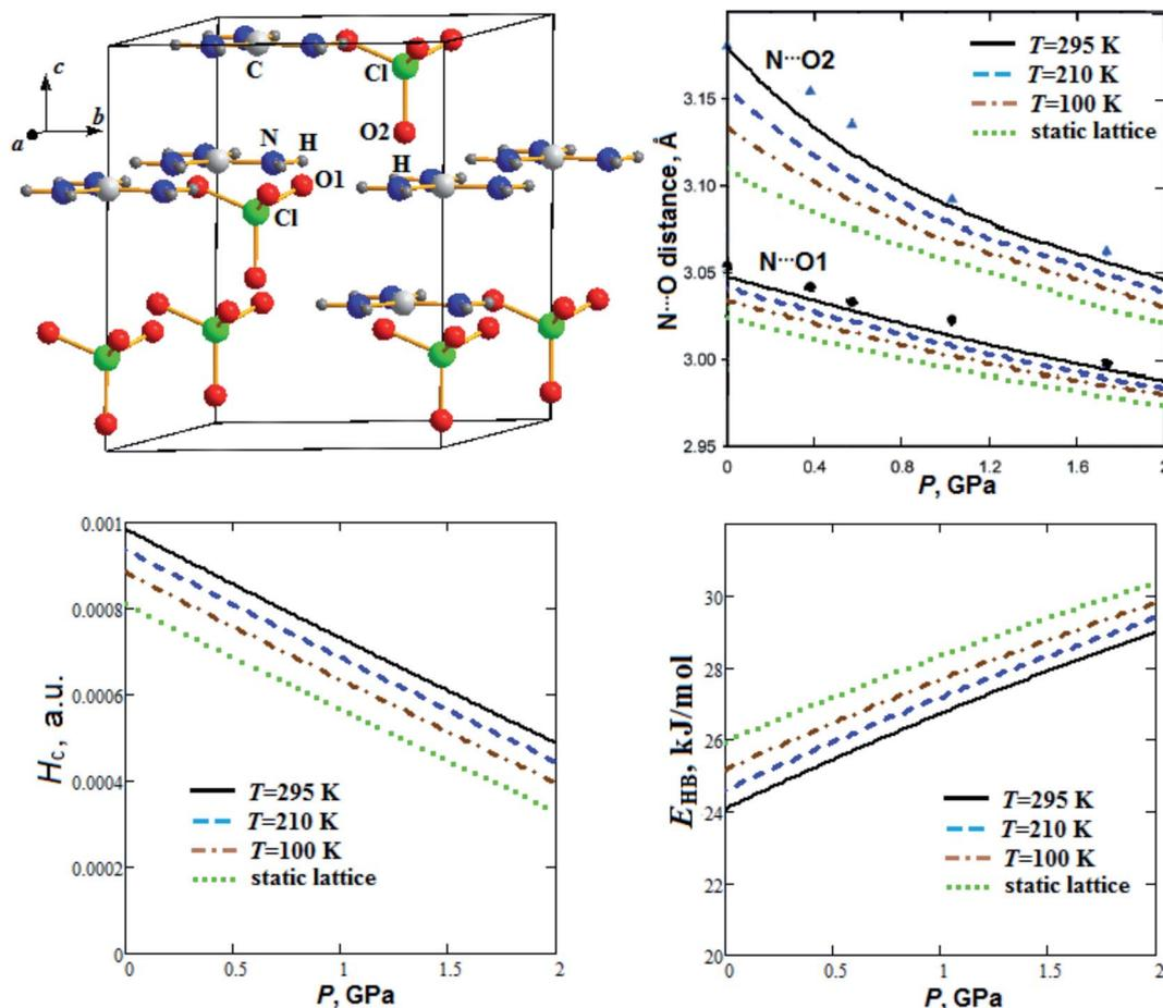
Fig. 3 Calculated semi-empirical pressure dependencies of N...O distances, energy density  $H_c$  at H...O1 critical points and hydrogen bond energy  $E_{HB}$  for guanidinium perchlorate at  $T = 295$  K (solid lines), 210 K (dashed lines), 100 K (dash-dotted lines) and at static lattice (dotted lines). Experimental points and triangles correspond to  $T = 295$  K.<sup>22</sup>
