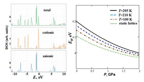
Fig. 7 Calculated anionic, cationic and total densities of states DOS (the energy of highest occupied states was set to zero), semi-empirical pressure dependencies of band gap  $E_g$  for guanidinium perchlorate at T = 295 K (solid lines), 210 K (dashed lines), 100 K (dash-dotted lines) and at static lattice (dotted lines).
