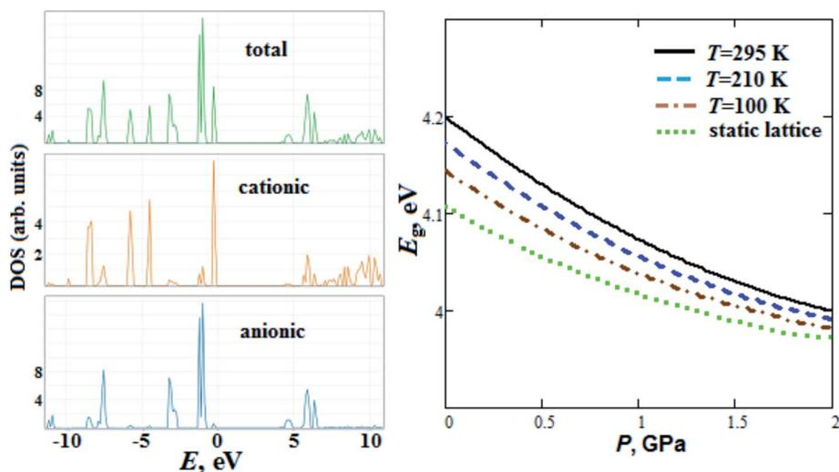
Fig. 7 Calculated anionic, cationic and total densities of states DOS (the energy of highest occupied states was set to zero), semi-empirical pressure dependencies of band gap  $E_g$  for guanidinium perchlorate at  $T = 295$  K (solid lines), 210 K (dashed lines), 100 K (dash-dotted lines) and at static lattice (dotted lines).
