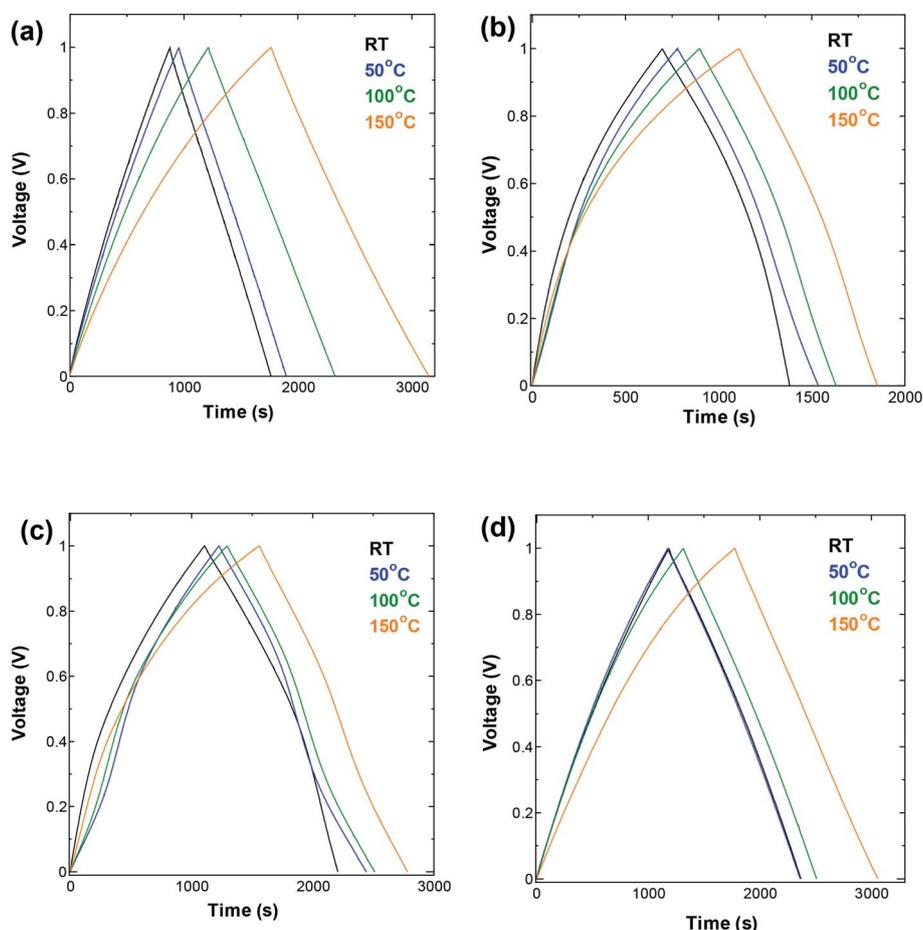
Fig. 3 GCD measurements performed at current density 10 mA g<sup>-1</sup> in a symmetric two-electrode cell using (a) SWCNT1.0 (b) SWCNT1.5 (c) SWCNT2.0, and (d) SWCNT5.0 as electrodes.
