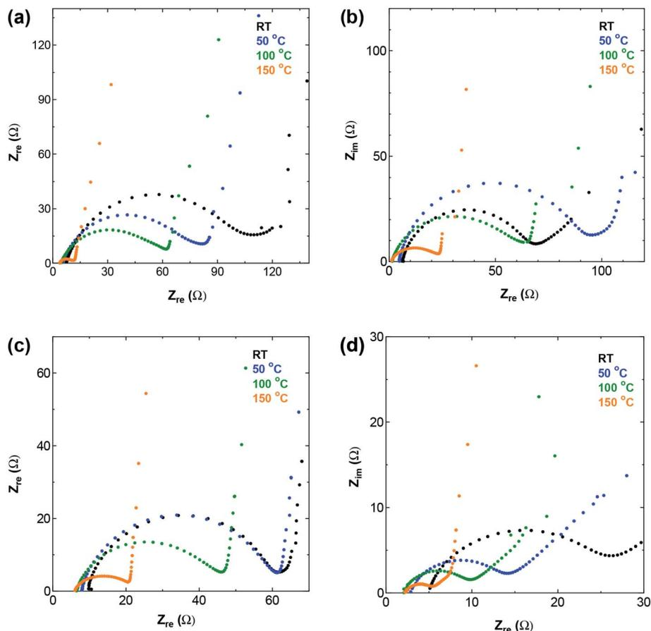
Fig. 5 The high and medium frequency region of Nyquist plot for (a) SWCNT1.0 (b) SWCNT1.5 (c) SWCNT2.0, and (d) SWCNT5.0 as electrodes.
