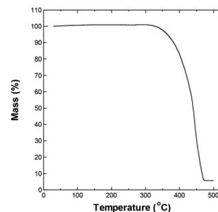
Fig. 1 TGA curve for P<sub>222(2O1)</sub>-TFSI measured with heating rate of 5 °C min<sup>-1</sup> under N<sub>2</sub> flow.
