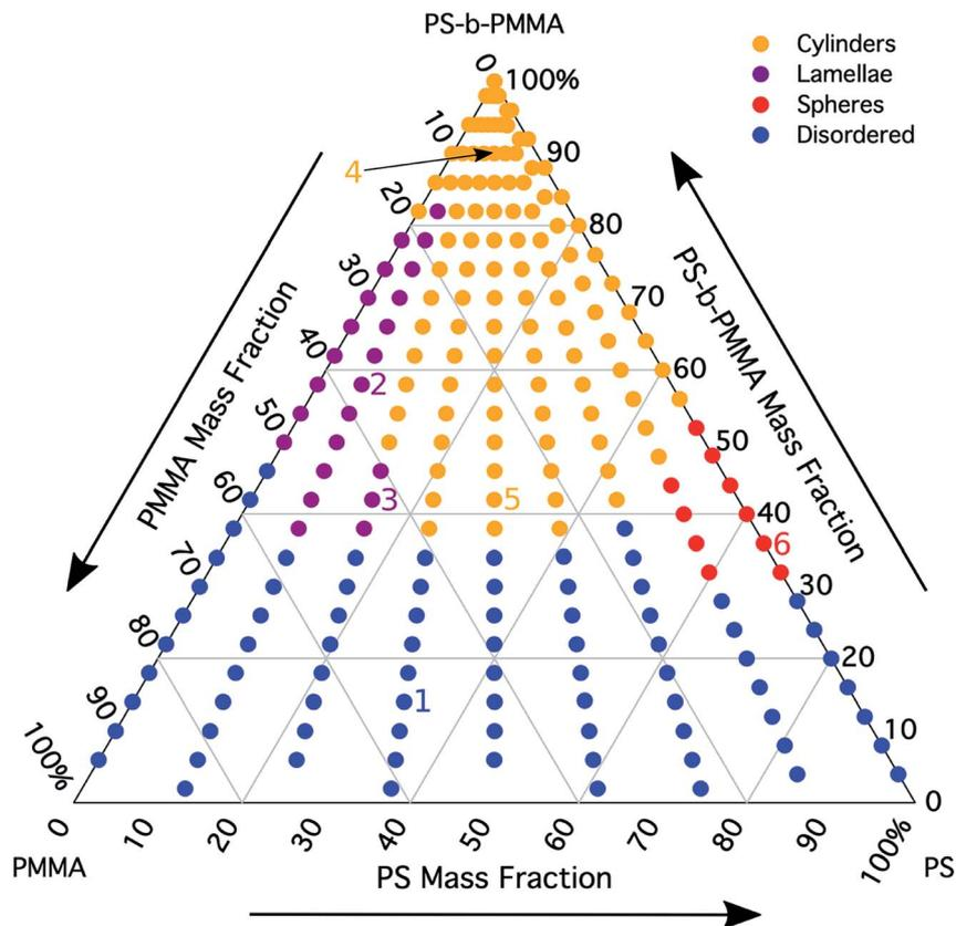
Fig. 2 Ternary morphology diagram constructed from ESD gradient samples for  $1.1 \text{ kg mol}^{-1}$  PMMA homopolymer,  $1.1 \text{ kg mol}^{-1}$  PS homopolymer, and  $67 \text{ kg mol}^{-1}$  PS-*b*-PMMA block copolymer. Cylindrical, lamellar, spherical, and disordered morphologies are identified. The numbered points correspond to exemplary cases that are elaborated on further in the main text.
