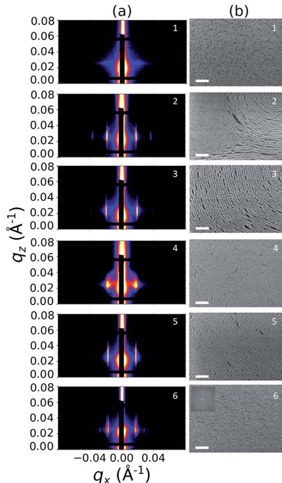
**Fig. 4** Structural characterization of selected points 1–6 in Fig. 2, including (a) GISAXS scattering patterns and (b) top view SEMs. The PMMA domains were selectively infiltrated with aluminum oxide to enhance image contrast for SEM analysis. All scale bars are 200 nm. The inset in (b) for point 6 is a Fourier power spectrum of that SEM.
