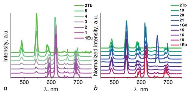
Fig. 5 Luminescence spectra for mixed metal samples in comparison with **1Eu**, **1Gd** and **2Tb** ones. (a) Emission spectra for Eu/Tb mixed metal series,  $\lambda_{\text{ex}} = 330$  nm. (b) Emission spectra for Eu/Tb/Gd mixed metal series,  $\lambda_{\text{ex}} = 330$  nm.
