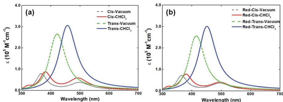
Fig. 3 Simulated absorption spectra of V-shaped azo-chromophore isomers (a) and their reduced version (b) in gas-phase and in  $\text{CHCl}_3$  solvent. The spectra were simulated using the information provided by TD-DFT and TD-DFT/PCM calculations for the eight lowest-energy transitions and by the superposition of individual Lorentzian lines (FWHM = 0.40 eV).
