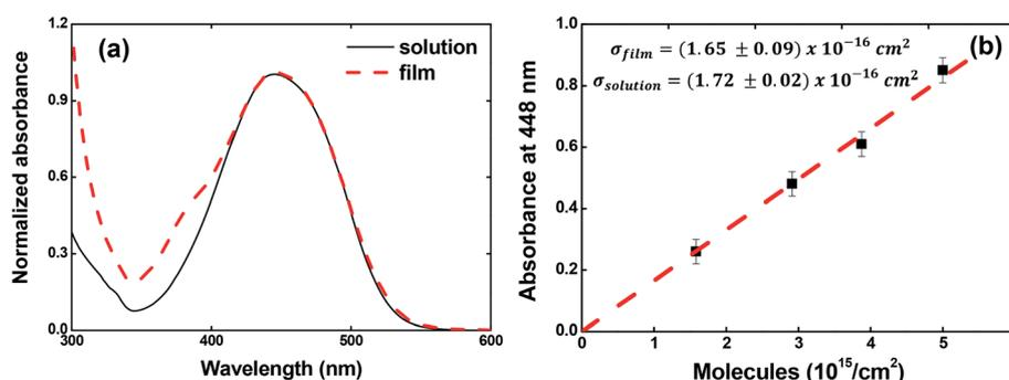
Fig. 2 (a) Absorption spectrum for V-shaped azo-chromophores/PMMA in chloroform solution (solid line) and guest–host film (dash line). (b) Absorbance at 448 nm as a function of the concentration.
