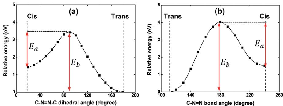
Fig. 4 The computed potential energy curve for thermal isomerization of V-shaped azo-chromophore molecule in gas-phase through the rotation (a) and inversion (b) mechanisms. The computed geometries of the *cis* and *trans* isomers and the transition state are also shown.  $E_b$  indicates the energy barrier of the thermal *trans*–*cis* isomerization and  $E_a$  indicates the activation energy of the kinetics of the thermal *cis*–*trans* isomerization.
