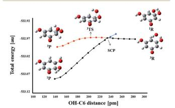
Fig. 8 Energy profiles for the RAF pathways of THB-O' with HO' in the singlet (blue line) and triplet (red line) states. The black line indicates the suggested reaction pathway. The spin crossing point (SCP) appears at the HO-C6 distance of 236.2 pm.
