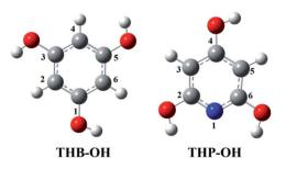
Fig. 1 Optimized geometries of the most stable rotamers of the investigated compounds in benzene. An atom labelling scheme is provided (grey – carbon atoms, white – hydrogen atoms, red – oxygen atoms, blue – nitrogen atoms).
