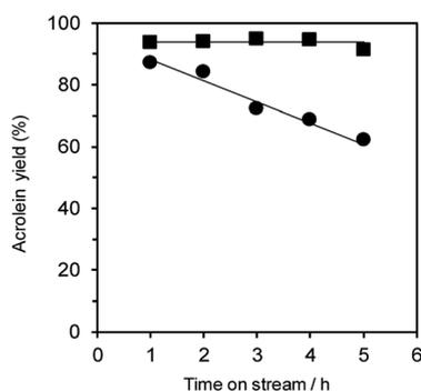
Fig. 5 Dehydration of glycerol to acrolein over WO<sub>3</sub>/Al<sub>2</sub>O<sub>3</sub> catalysts with 20 wt% WO<sub>3</sub> loading and under flowing N<sub>2</sub> (circle) and O<sub>2</sub> (square). Conditions: catalyst (100 mg), WHSV by glycerol (4.7 h<sup>-1</sup>), T = 588 K.
