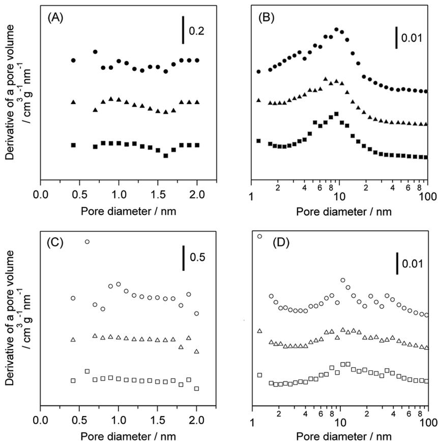
Fig. 6 Pore size distribution of the (A) micropore and (B) mesopore regions in  $\text{WO}_3/\text{Al}_2\text{O}_3$  with 20 wt%  $\text{WO}_3$  loading and (C) micropore and (D) mesopore regions in H-ZSM-5(90). Fresh catalyst (circle), after the reaction with  $\text{N}_2$  (triangle) and  $\text{O}_2$  (square) for 5 h.
