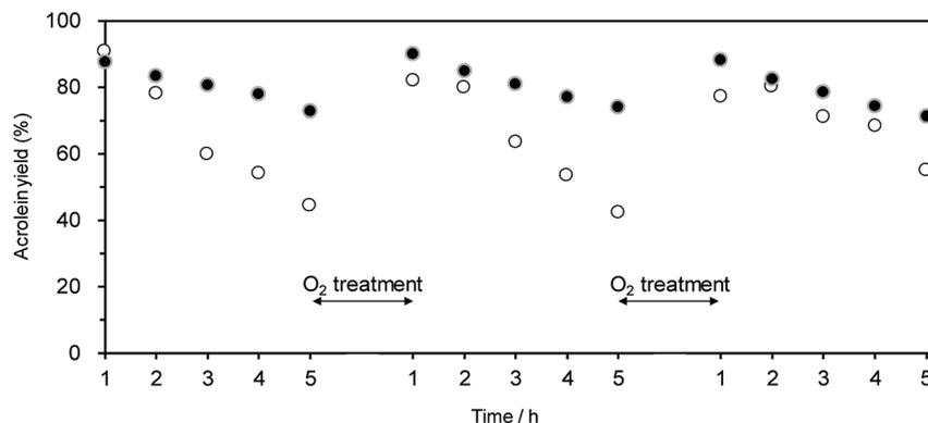
Fig. 4 Effect of O<sub>2</sub> treatment on acrolein yield over (●) WO<sub>3</sub>/Al<sub>2</sub>O<sub>3</sub> with 20 wt% WO<sub>3</sub> loading and (○) H-ZSM-5(90) catalysts. Conditions: catalyst (100 mg), WHSV by glycerol (4.7 h<sup>-1</sup>), T = 588 K. O<sub>2</sub> treatment was carried out after 5 h at the temperature at which deposited coke completely decomposed; 823 K (WO<sub>3</sub>/Al<sub>2</sub>O<sub>3</sub>) and 923 K (H-ZSM-5), respectively.
