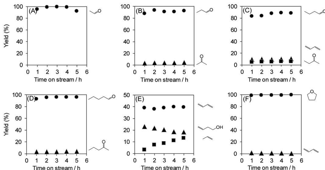
Fig. 7 Dehydration of various polyols over  $\text{WO}_3/\text{Al}_2\text{O}_3$  catalysts with 20 wt%  $\text{WO}_3$  loading. Conditions: catalyst (100 mg), WHSV by substrate ( $4.7 \text{ h}^{-1}$ ),  $T = 588 \text{ K}$ . (A) Ethylene glycol, (B) 1,2-propanediol, (C) 1,2-butanediol, (D) 1,2-pentanediol, (E) 1,3-butanediol and (F) 1,4-butanediol.
