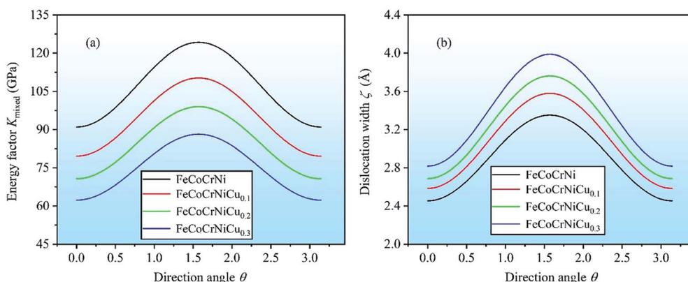
Fig. 9 Variation curves of (a) energy factor  $K_{\text{mixed}}$  and (b) dislocation width  $\zeta$  versus direction angle  $\theta$  ( $0 \leq \theta \leq \pi$ ) between Burgers vector and dislocation line.
