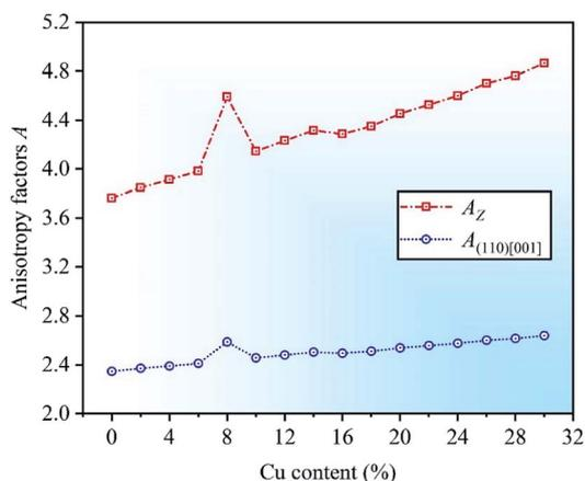
Fig. 7 Calculated anisotropy factors  $A$  as a function of Cu content for CrFeCoNiCu<sub>x</sub> ( $0 \leq x \leq 0.3$ ) HEAs.
