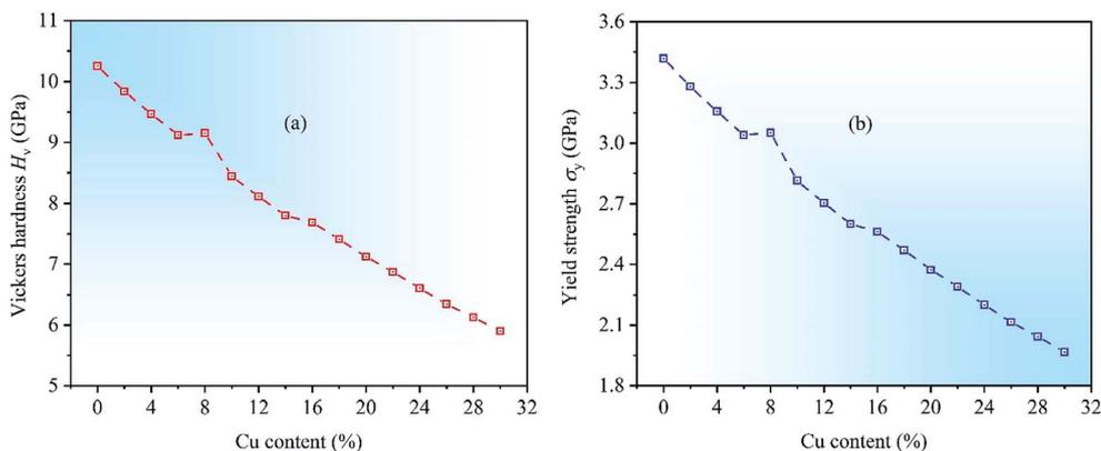
Fig. 6 Calculated (a) Vickers hardness  $H_v$  and (b) yield strength  $\sigma_y$  as a function of Cu content for CrFeCoNiCu<sub>x</sub> ( $0 \leq x \leq 0.3$ ) HEAs.
