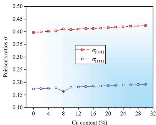
Fig. 5 Calculated Poisson's ratios  $\sigma$  as a function of Cu content for CrFeCoNiCu<sub>x</sub> ( $0 \leq x \leq 0.3$ ) HEAs.
