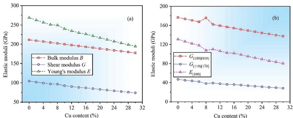
Fig. 3 Calculated (a) and (b) elastic moduli as a function of Cu content for CrFeCoNiCu<sub>x</sub> ( $0 \leq x \leq 0.3$ ) HEAs.
