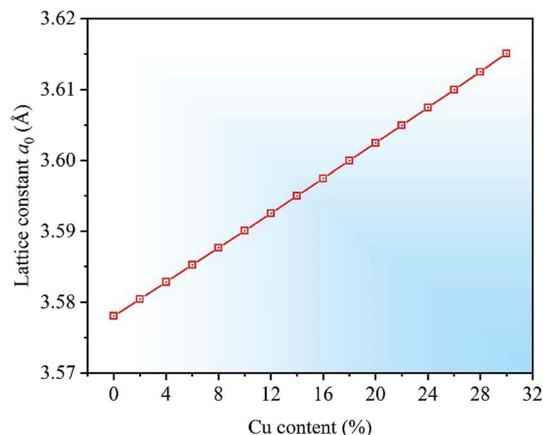
Fig. 1 Calculated lattice constant *a*<sub>0</sub> as a function of Cu content for CrFeCoNiCu<sub>x</sub> (0 ≤ *x* ≤ 0.3) HEAs.
