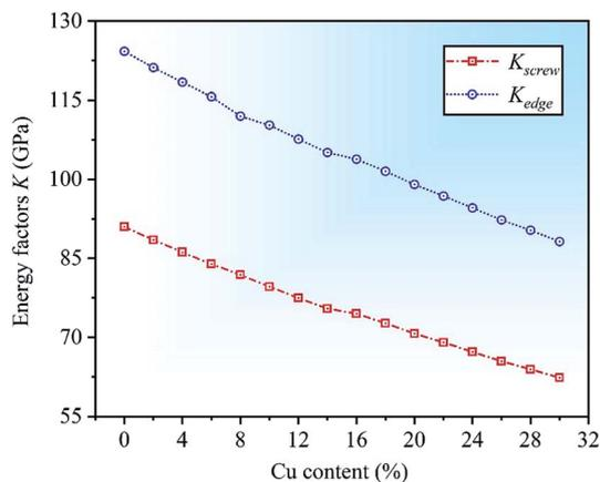
Fig. 8 Calculated energy factors  $K$  as a function of Cu content for CrFeCoNiCu<sub>*x*</sub> ( $0 \leq x \leq 0.3$ ) HEAs.
