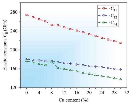
Fig. 2 Calculated elastic constants  $C_{ij}$  as a function of Cu content for CrFeCoNiCu<sub>x</sub> ( $0 \leq x \leq 0.3$ ) HEAs.
