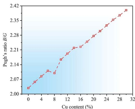
Fig. 4 Calculated Pugh's ratio  $B/G$  as a function of Cu content for CrFeCoNiCu<sub>x</sub> ( $0 \leq x \leq 0.3$ ) HEAs.
