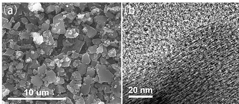
Fig. 1 (a) SEM and (b) TEM images of microporous carbon.
