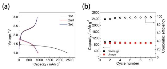
Fig. 2 Charge/discharge profile (a) and cycle performance (b) of the microporous carbon-supported sulfur cathode.
