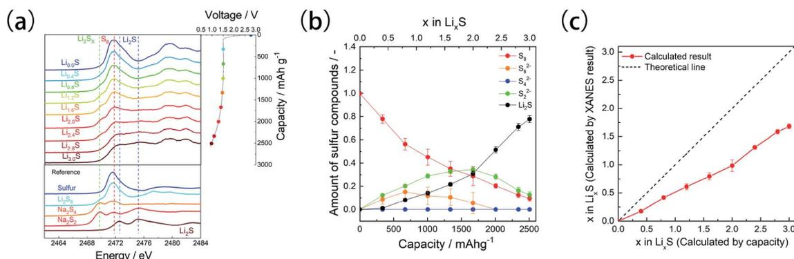
Fig. 4 (a) Sulfur K-edge XANES spectra obtained from the *operando* XAS measurements of the microporous carbon-supported sulfur cathode. (b) Sulfur compound ratio of the microporous carbon-supported sulfur cathode during the first discharge, calculated by the linear combination fitting (LCF) analysis of XANES spectra. (c) Lithium compositions calculated from the LCF analysis and electrochemical capacity data.
