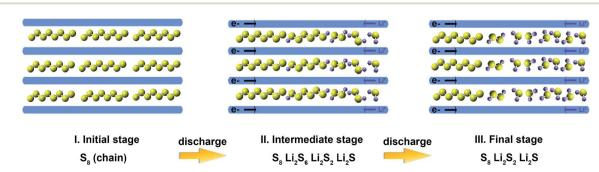
Fig. 5 Reaction model for the microporous carbon-supported sulfur cathodes.
