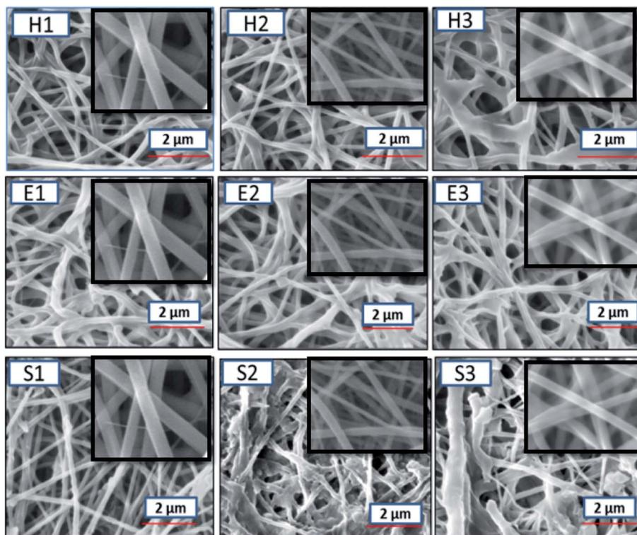
Fig. 7 E-SEM images of the degraded nanofiber mats (1) PCL-13, (2) PP-133 and (3) PP-1335 (inset shows the E-SEM images of non-degraded nanofibers) where H – hydrolytic degradation, E – enzymatic degradation and S – degradation in soil.
