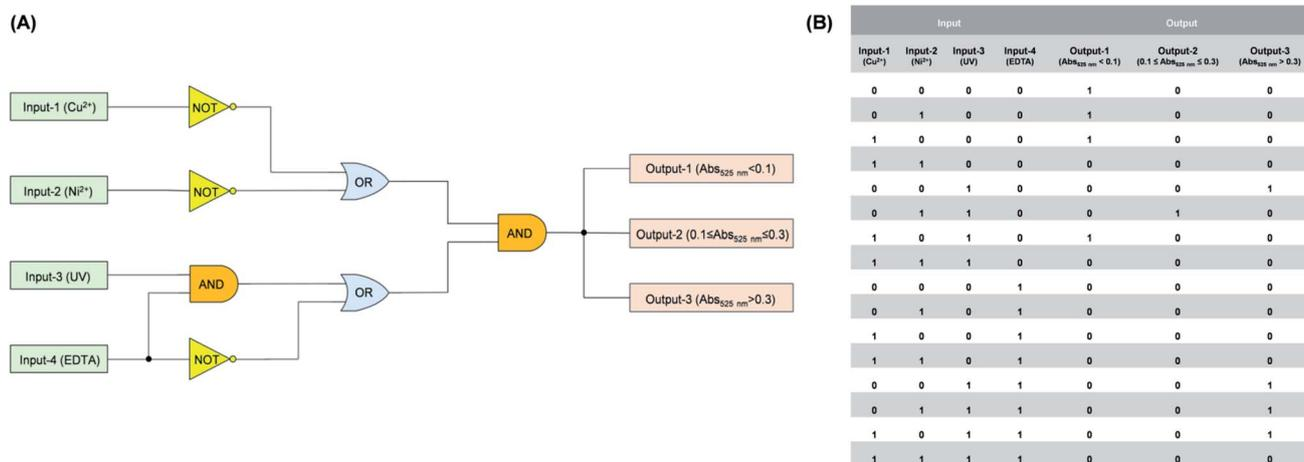
Fig. 5 (A) A logic circuit with four inputs and three outputs: input-1 (Cu<sup>2+</sup> addition), input-2 (Ni<sup>2+</sup> addition), input-3 (UV light irradiation), input-4 (EDTA addition), output-1 (absorbance at 525 nm < 0.1), output-2 (0.1 ≤ absorbance at 525 nm ≤ 0.3), output-3 (absorbance at 525 nm > 0.3). (B) Truth table for the molecular logic circuit.
