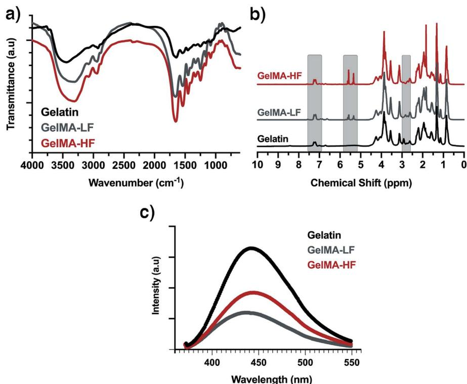
Fig. 2 Characterization of gelatin and methacrylated gelatin: (a) FTIR, (b) <sup>1</sup>H-NMR, (c) fluorescence spectra (the gelatin and GelMA concentrations are 0.5 mg mL<sup>-1</sup>).
