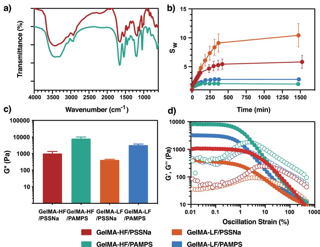
Fig. 3 Characterization of the polyelectrolyte-grafted GelMA hydrogel: (a) representative FTIR spectra of GelMA-HF/PSSNa and GelMA-HF/PAMPS, (b) swelling behavior (pH 7.4,  $20^\circ\text{C}$ ), (c) complex modulus (gap  $1000\ \mu\text{m}$ , determined at a strain of 0.01% and temperature of  $25^\circ\text{C}$ ), and (d) oscillatory shear strain assays (gap  $1000\ \mu\text{m}$ ,  $25^\circ\text{C}$ ).
