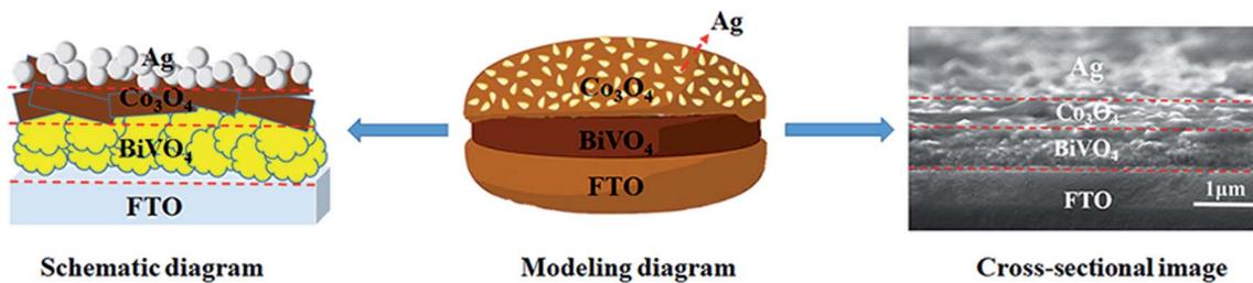
Fig. 1 Schematic diagram, modeling diagram and cross-sectional image of triadic Ag/Co<sub>3</sub>O<sub>4</sub>/BiVO<sub>4</sub> photoanode.
