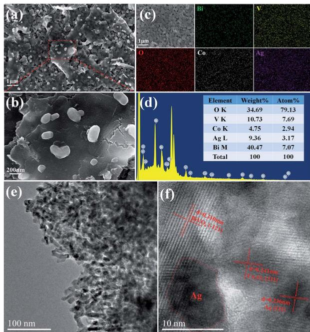
Fig. 5 SEM images (a and b) of Ag/Co<sub>3</sub>O<sub>4</sub>/BiVO<sub>4</sub>, EDX mappings (c and d) for Ag/Co<sub>3</sub>O<sub>4</sub>/BiVO<sub>4</sub>, TEM (e) and HRTEM (f) images of Ag/Co<sub>3</sub>O<sub>4</sub>/BiVO<sub>4</sub>.
