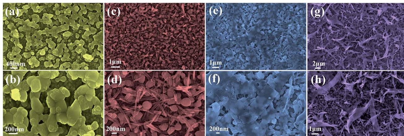
Fig. 6 SEM images (a and b) of 1 mM Co<sub>3</sub>O<sub>4</sub>/BiVO<sub>4</sub>; (c and d) of 2 mM Co<sub>3</sub>O<sub>4</sub>/BiVO<sub>4</sub>; (e and f) of 3 mM Co<sub>3</sub>O<sub>4</sub>/BiVO<sub>4</sub>; (g and h) of 4 mM Co<sub>3</sub>O<sub>4</sub>/BiVO<sub>4</sub>.
