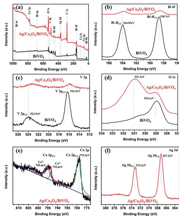
Fig. 4 XPS survey spectra of pristine  $\text{BiVO}_4$  and  $\text{Ag}/\text{Co}_3\text{O}_4/\text{BiVO}_4$ : (a) survey scan; (b) Bi 4f; (c) V 2p; and (d) O 1s. (e) Co 2p and (f) Ag 3d scan spectra of  $\text{Ag}/\text{Co}_3\text{O}_4/\text{BiVO}_4$ .
