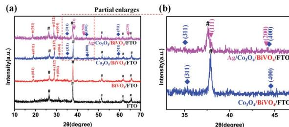
Fig. 3 (a) XRD patterns of FTO,  $\text{BiVO}_4/\text{FTO}$ ,  $\text{Co}_3\text{O}_4/\text{BiVO}_4/\text{FTO}$  and  $\text{Ag}/\text{Co}_3\text{O}_4/\text{BiVO}_4/\text{FTO}$ . (b) Enlarged view of the area marked with the red dots in the (a) XRD patterns.
