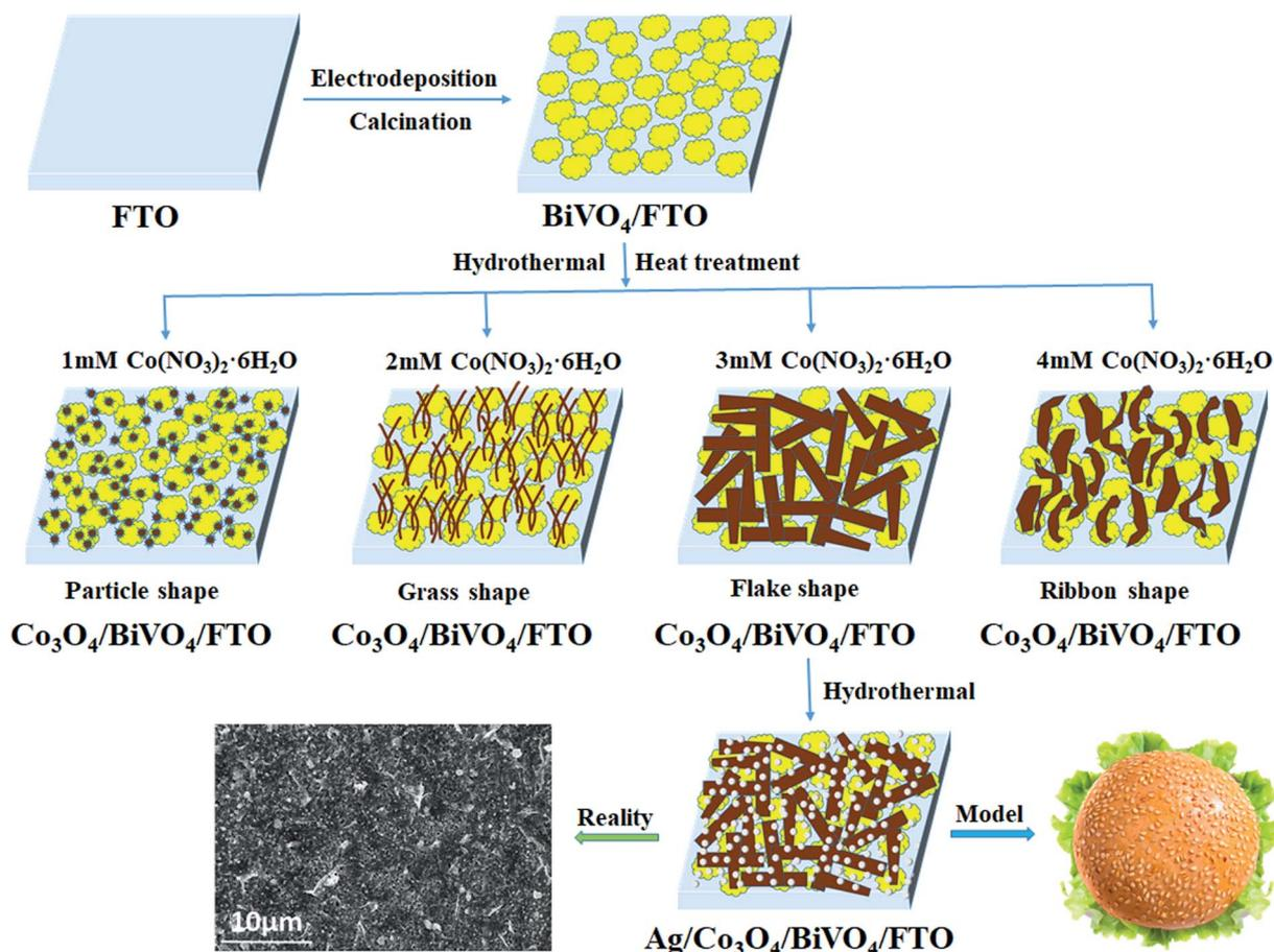
Fig. 2 Synthetic procedure of triadic Ag/Co<sub>3</sub>O<sub>4</sub>/BiVO<sub>4</sub> photoanode.
