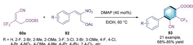
Scheme 24 DMAP-catalyzed [4 + 2] benzannulation to synthesize penta-substituted benzenes.
