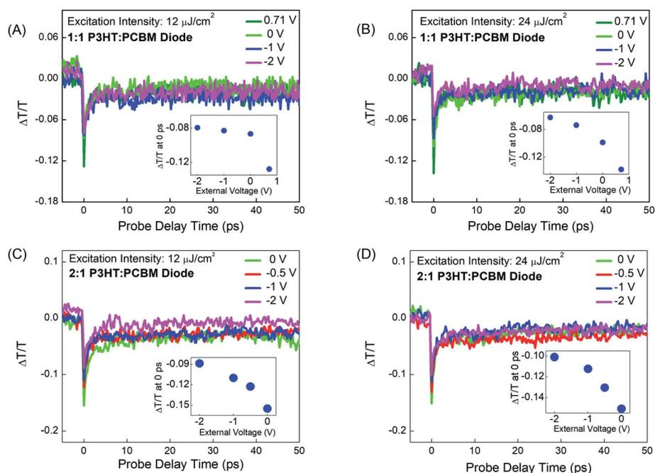
Fig. 3 Differential probe pulse transmission dynamics  $\Delta T/T$  showing photoinduced transient absorption at 638 nm in 1 : 1 (top panels) and 2 : 1 (bottom panels) P3HT:PCBM solar cell devices after initial pump pulse excitation fluences of 12 (left panels) and 24  $\mu\text{J cm}^{-2}$  (right panels) and for different applied voltages.
