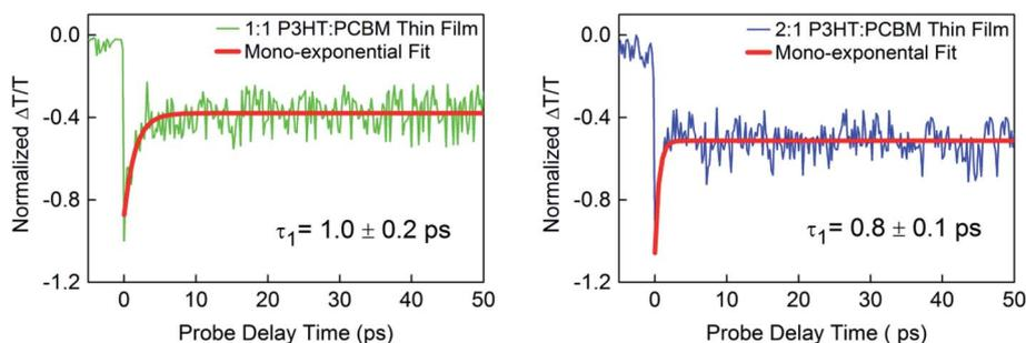
**Fig. 2** Normalized differential probe pulse transmission dynamics  $\Delta T/T$  showing photoinduced transient absorption at 638 nm in P3HT:PCBM thin films with weight ratios 1 : 1 and 2 : 1 using  $12 \mu\text{J cm}^{-2}$  initial pump pulse excitation at 520 nm.
