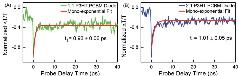
Fig. 4 Differential probe transmission dynamics  $\Delta T/T$  showing photoinduced transient absorption at 638 nm in 1 : 1 (A) and 2 : 1 (B) P3HT:PCBM solar cell devices under a forward bias compensating the built-in potential after initial pump pulse excitation with  $24 \mu\text{J cm}^{-2}$ .
