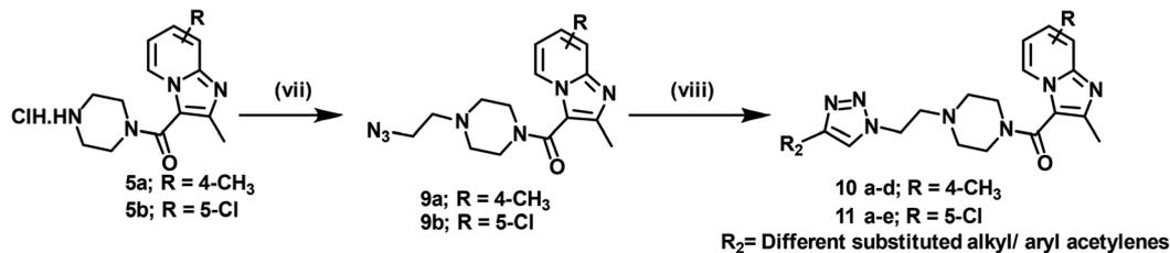
**Scheme 3** Preparation of title compounds **10a–d** and **11a–e**. Reagents and conditions: (vii) **5a/5b** (1.0 eq.), 2-azidoethyl 4-methylbenzenesulfonate (1.5 eq.), K<sub>2</sub>CO<sub>3</sub> (4 eq.), DMF, 100 °C, 12 h; (viii) substituted terminal alkynes (1.5 eq.), CuSO<sub>4</sub>·5H<sub>2</sub>O, (10 mol%), sodium ascorbate (10 mol%), DMF : water (8 : 2), rt, 7–12 h.
