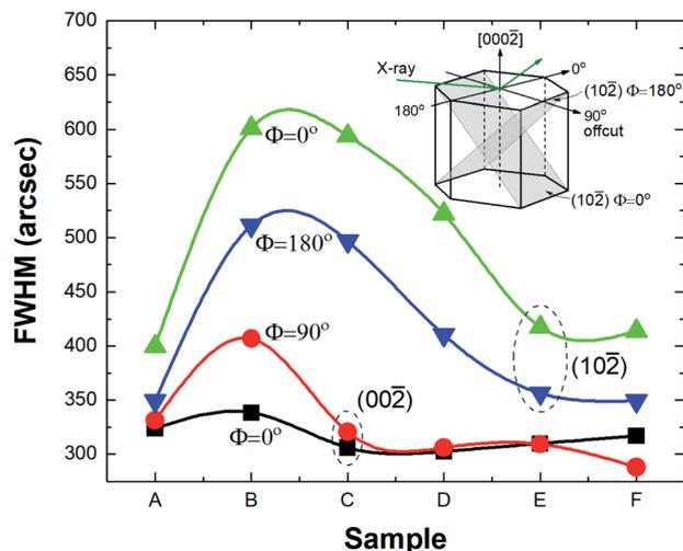
Fig. 3 The minimum and maximum FWHMs of GaN $(00\bar{2})$  and GaN $(10\bar{2})$  RCs measured at different  $\Phi$  values. The inset illustrates the XRD optical alignment with respect to the GaN crystal geometry.
