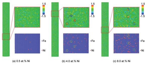
Fig. 2 Local atomic pressure maps of Fe-Ni alloy nanowires with different Ni content (annealing at 300 K), (a) 0.5 at%, (b) 4.0 at% and (c) 8.0 at%. Atoms are colored according to the local atomic pressure. Pressures are given in GPa. The corresponding composition maps are shown in the below insert schematic. Fe: blue atoms. Ni: red atoms.
