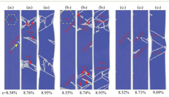
Fig. 4 The atomic configuration of Fe-Ni alloy nanowires under different strain at 1 K. (a) 0.5 at% Ni, (b) 5.0 at% Ni, (c) 8.0 at% Ni.
