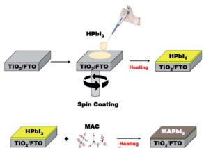
Fig. 4 Schematic illustration of the formation of MAPbI $_3$  film. Fabrication of HPbI $_3$  film on a TiO $_2$ /FTO substrate was achieved by the spin-coating method (top panel). Conversion of HPbI $_3$  film to MAPbI $_3$  film using MAC, where the vapor-phase reaction was performed in an autoclave reactor filled with the MAC powder (bottom panel).
