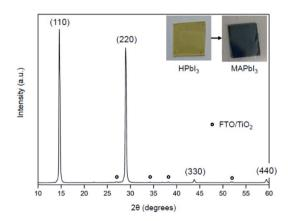
Fig. 5 XRD patterns of the MAPbI $_3$  film converted from the HPbI $_3$  film via vapor-phase reaction using MAC. Asterisk marks indicate diffraction peaks of TiO $_2$ /FTO. The inset shows photographs of HPbI $_3$  (left) and MAPbI $_3$  (right) films. The images were taken before (left) and after (right) the reaction between HPbI $_3$  and MAC.
