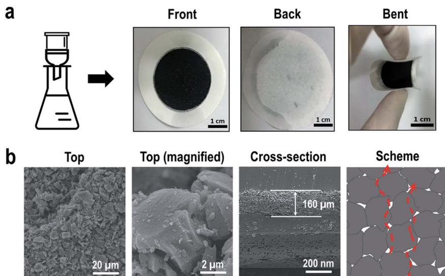
**Fig. 1** (a) Photographs of ACLA-C photothermal layer (front, back, and bent) and (b) SEM images of ACLA-C (top, cross-section) with the scheme exhibiting the formation of intraparticle pores through which mass transport occurs.
