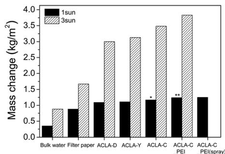
Fig. 5 Summary of water evaporation rates by solar-to-steam generation measured for 1 h under 1 and 3 sun irradiance.
