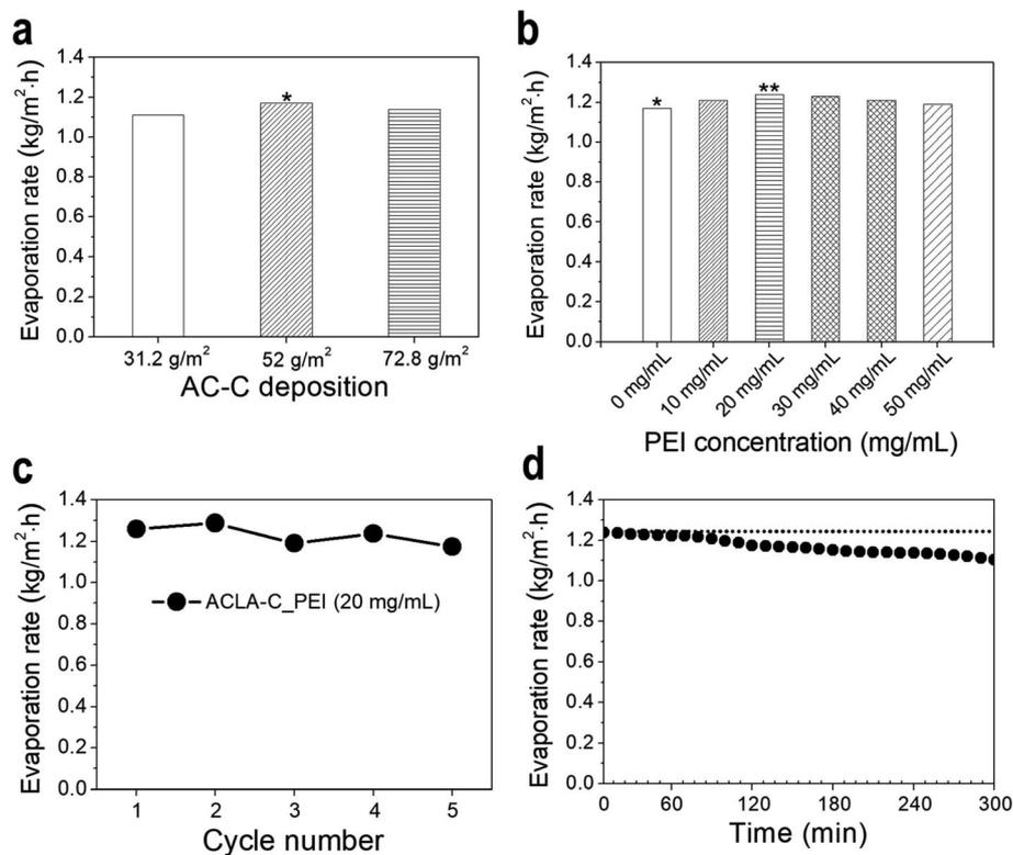
Fig. 3 Mass change in water by solar-to-steam generation for (a) ACLA-C with different loading amounts of AC-C, and (b) ACLA-C<sub>PEI</sub> with different concentration of PEI polymer. (c) The cyclic test with drying samples after each measurement using ACLA-C (20 mg mL<sup>-1</sup>). (d) The time-on-stream evaporation rate of salt water by ACLA-C (20 mg mL<sup>-1</sup>). All the measurements are performed under the irradiance of 1 sun for 1 h.
