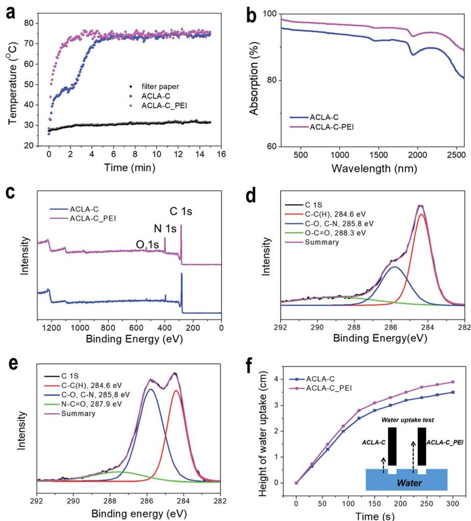
Fig. 4 (a) Surface temperature profiles of ACLA-C and ACLA-C<sub>PEI</sub> photothermal layers in dry condition. (b) Absorption spectra of ACLA-C and ACLA-C<sub>PEI</sub> measured in dry state. (c) XPS survey scan of ACLA-C and ACLA-C<sub>PEI</sub>. High-resolution C 1s spectra of (d) ACLA-C and (e) ACLA-C<sub>PEI</sub>, (f) water uptake measurements of ACLA-C and ACLA-C<sub>PEI</sub> with respect to time.
