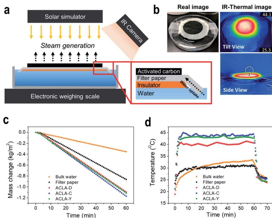
**Fig. 2** (a) Schematic illustration of the lab-scaled experimental setup for solar-to-steam generation, (b) real image and IR thermal images of the photothermal layer in the wet condition under 1 sun, (c) mass change profile by solar-to-steam generation for 1 h under 1 sun and, (d) temperature profiles of bulk-water, bare filter paper, and three commercial AC-based photothermal layers during solar-to-steam generation under 1 sun.
