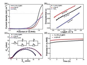
Fig. 5 (a) LSV curves of  $O_V$ -HCo $_3$ O $_4$ @NC, A-ZIF-67 and RuO $_2$ . (b) Corresponding Tafel plots. (c) Nyquist plots of  $O_V$ -HCo $_3$ O $_4$ @NC and A-ZIF-67 at a potential of 1.57 V vs. RHE; the inset is the equivalent electrical circuit used to model the OER kinetics process. (d) Chronopotentiometry measurements for  $O_V$ -HCo $_3$ O $_4$ @NC and A-ZIF-67 in OER.
