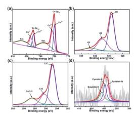
Fig. 4 XPS spectra of  $O_V$ -HCO $_3O_4$ @NC in the (a) Co 2p, (b) O 1s, (c) C 1s, and (d) N 1s regions.
