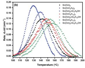
Fig. 10 Plots of (a) monomer conversion ( $\alpha$ ) and (b) rate (d $\alpha$ /dt) against temperature (°C) for L-lactide ring-opening polymerization using various initiators/initiating systems at a heating rate of 5 °C min<sup>-1</sup>.
