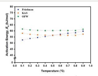
Fig. 9 Dependence of activation energy ( $E_a$ , kJ mol $^{-1}$ ) on the fraction of conversion ( $\alpha$ ) from the data obtained from the: ( $\blacksquare$ ) Friedman; ( $\bullet$ ) KAS; and ( $\bullet$ ) OFW isoconversional methods for the ROP of L-lactide using 1.0 mol% liquid Sn(O $nC_4H_9$ ) $_2$  as an initiator.
