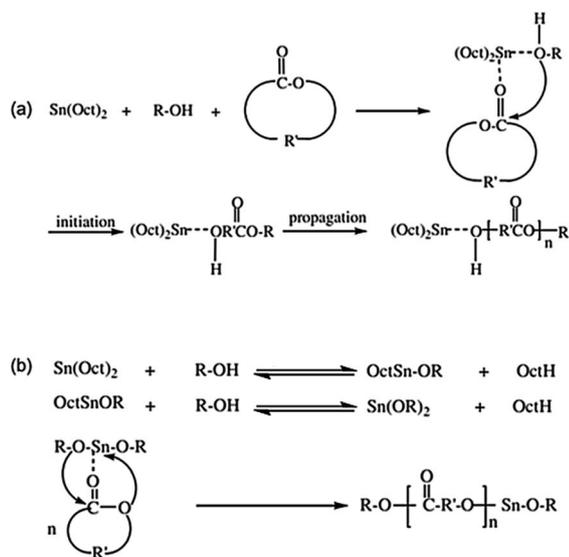
Fig. 1 Comparison of the old (a) and the new (b) mechanistic proposals using  $\text{Sn}(\text{Oct})_2$ : (a) complexation of the monomer and alcohol prior to ROP and (b) formation of tin(II) alkoxide before ROP.<sup>13,14</sup>
