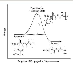
Fig. 11 Visualization of the meaning of the value of activation energy,  $\textit{E}_{\text{a}}$ .
