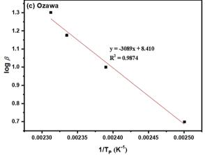
Fig. 6  $E_a$  determinations based on dynamic methods of: (a) Kissinger; (b) Flynn–Wall; and (c) Ozawa for the ROP of L-lactide using 1.0 mol% liquid  $Sn(OnC_4H_9)_2$  as an initiator.
