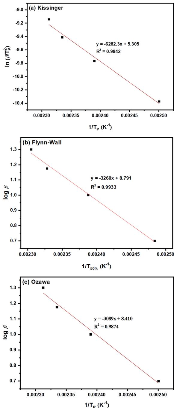
Fig. 6  $E_a$  determinations based on dynamic methods of: (a) Kissinger; (b) Flynn–Wall; and (c) Ozawa for the ROP of L-lactide using 1.0 mol% liquid  $\text{Sn}(\text{OnC}_4\text{H}_9)_2$  as an initiator.
