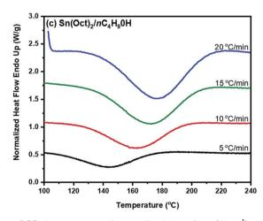
Fig. 5 DSC thermograms of normalized heat flow (W g $^{-1}$ ) against temperature (°C) for the ROP of L-lactide using: (a) 1.0 mol% Sn(Oct) $_2$ ; (b) 1.0 mol% liquid Sn(OnC $_4$ H $_9$ ) $_2$ ; and (c) 1.0/2.0 mol% Sn(Oct) $_2$ /  $nC_4$ H $_9$ OH as initiators and initiating system at heating rates of (–) 5, (–) 10, (–) 15, and (–) 20 °C min $^{-1}$ .
