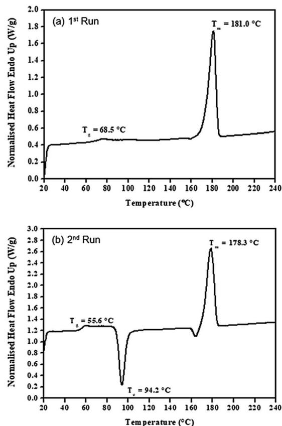
Fig. 12 DSC thermograms for (a) 1<sup>st</sup> run and (b) 2<sup>nd</sup> run of the purified poly(L-lactide) (PLLA 1) using 0.01 mol% liquid Sn(OnC<sub>4</sub>H<sub>9</sub>)<sub>2</sub> as an initiator at 100 °C for 24 h.
