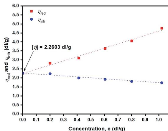
**Fig. 13** Plots of reduced viscosity,  $\eta_{\text{red}}$  (■) and inherent viscosity,  $\eta_{\text{inh}}$  (●) in  $\text{CHCl}_3$  at  $25 \pm 0.1$   $^\circ\text{C}$  against concentration (g dL<sup>-1</sup>) for purified poly( $L$ -lactide) (PLLA 9) obtained from using 0.05 mol% liquid  $\text{Sn}(\text{OnC}_4\text{H}_9)_2$  as an initiator at  $120$   $^\circ\text{C}$  for 24 h.
