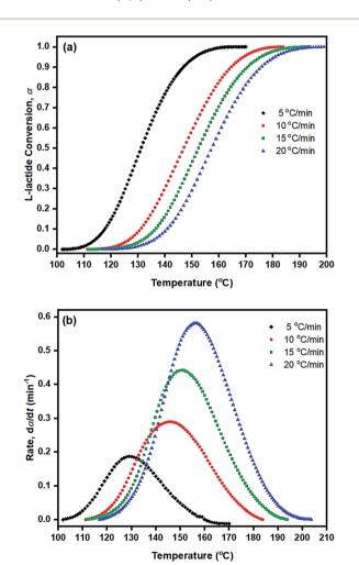
Fig. 7 Plots of (a) fraction of conversion ( $\alpha$ ) and (b) rate of polymerization (d $\alpha$ /dt, min $^{-1}$ ) against temperature (°C) for the ROP of L-lactide using 1.0 mol% liquid Sn(OnC<sub>4</sub>H<sub>9</sub>)<sub>2</sub> as an initiator at heating rates of: ( $\bullet$ ) 5; ( $\bullet$ ) 10; ( $\bullet$ ) 15; and ( $\bullet$ ) 20 °C min $^{-1}$ .
