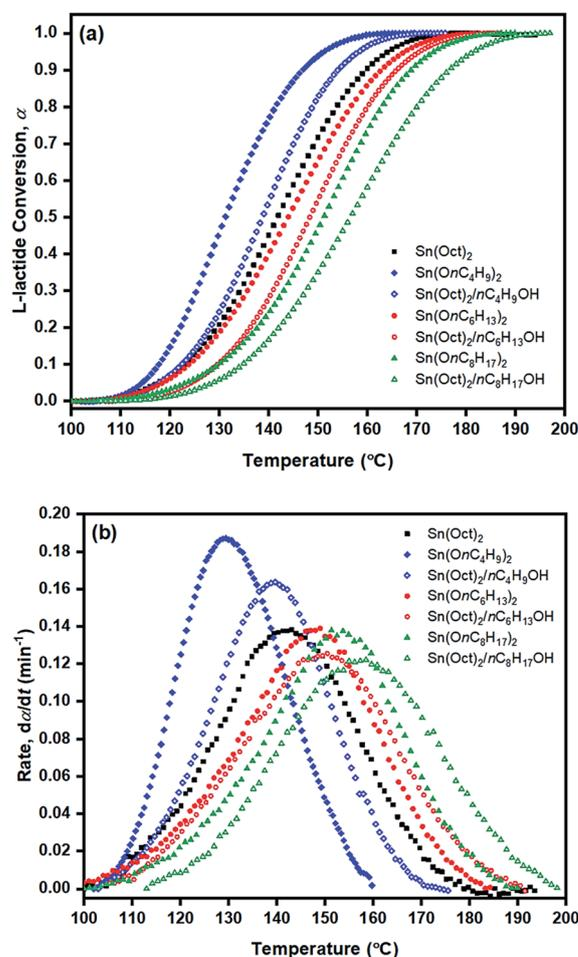
**Fig. 10** Plots of (a) monomer conversion ( $\alpha$ ) and (b) rate ( $d\alpha/dt$ ) against temperature (°C) for L-lactide ring-opening polymerization using various initiators/initiating systems at a heating rate of 5 °C min<sup>-1</sup>.
