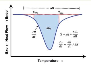
Fig. 4 Idealized DSC curve for kinetic parameters determination by using Borchardt and Daniels (B/D) method.
