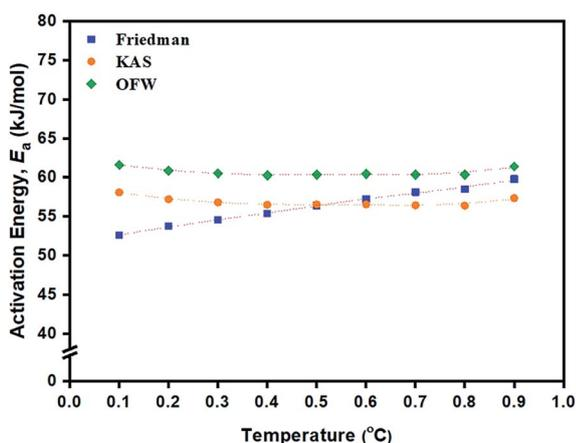
**Fig. 9** Dependence of activation energy ( $E_a$ , kJ mol<sup>-1</sup>) on the fraction of conversion ( $\alpha$ ) from the data obtained from the: (■) Friedman; (●) KAS; and (◆) OFW isoconversional methods for the ROP of L-lactide using 1.0 mol% liquid Sn(OnC<sub>4</sub>H<sub>9</sub>)<sub>2</sub> as an initiator.
