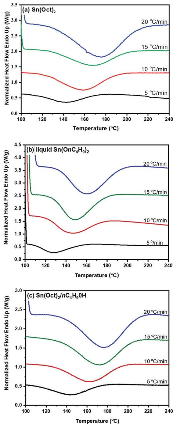
**Fig. 5** DSC thermograms of normalized heat flow ( $\text{W g}^{-1}$ ) against temperature ( $^{\circ}\text{C}$ ) for the ROP of L-lactide using: (a) 1.0 mol%  $\text{Sn}(\text{Oct})_2$ ; (b) 1.0 mol% liquid  $\text{Sn}(\text{OnC}_4\text{H}_9)_2$ ; and (c) 1.0/2.0 mol%  $\text{Sn}(\text{Oct})_2/n\text{C}_4\text{H}_9\text{OH}$  as initiators and initiating system at heating rates of (—) 5, (—) 10, (—) 15, and (—) 20  $^{\circ}\text{C min}^{-1}$ .
