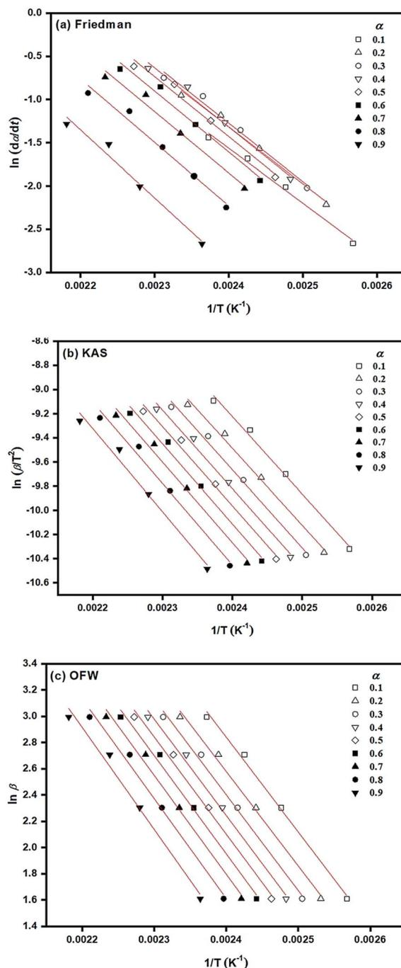
Fig. 8 Determination of  $E_a$  based on isoconversional methods of: (a) Friedman; (b) KAS; and (c) OFW for the ROP of L-lactide using 1.0 mol% liquid  $\text{Sn}(\text{OnC}_4\text{H}_9)_2$  as an initiator.
