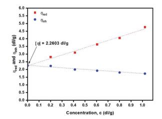
Fig. 13 Plots of reduced viscosity,  $\eta_{\rm red}$  ( $\blacksquare$ ) and inherent viscosity,  $\eta_{\rm inh}$  ( $\bullet$ ) in CHCl<sub>3</sub> at 25  $\pm$  0.1 °C against concentration (g dL<sup>-1</sup>) for purified poly(L-lactide) (PLLA 9) obtained from using 0.05 mol% liquid Sn(OnC<sub>4</sub>H<sub>9</sub>)<sub>2</sub> as an initiator at 120 °C for 24 h.
