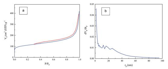
Fig. 4 (a) N<sub>2</sub> adsorption-desorption isotherm and (b) pore size distribution of CA powder.
