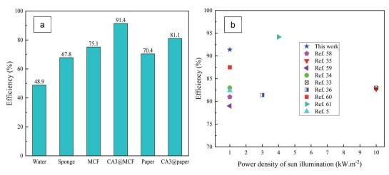
Fig. 11 (a) The efficiency of water (without absorbent), sponge, substrates and absorbent layers, (b) comparison of the efficiency in literatures to this work
