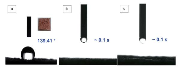
Fig. 8 The water contact angle of (a) hydrophobic CF, (b) MCF substrate, (c) CA3@MCF membrane (the videos and figures of the water droplet absorption by MCF (Video S1†), CA3@MCF (Video S2†), paper (Fig. S4a†) and CA3@paper (Fig. S4b†) samples are available in ESI†).
