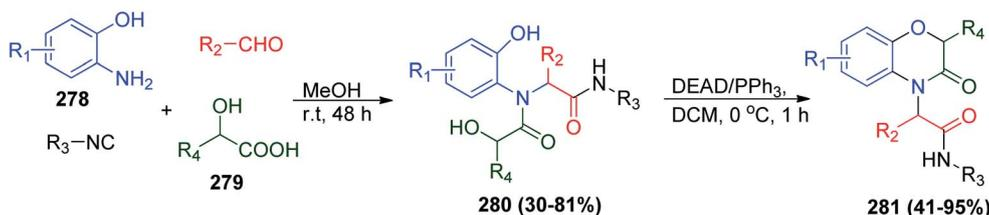
Scheme 59 Synthesis of benzoxazinones **281** via U-4CR/Mitsunobu cyclization.
