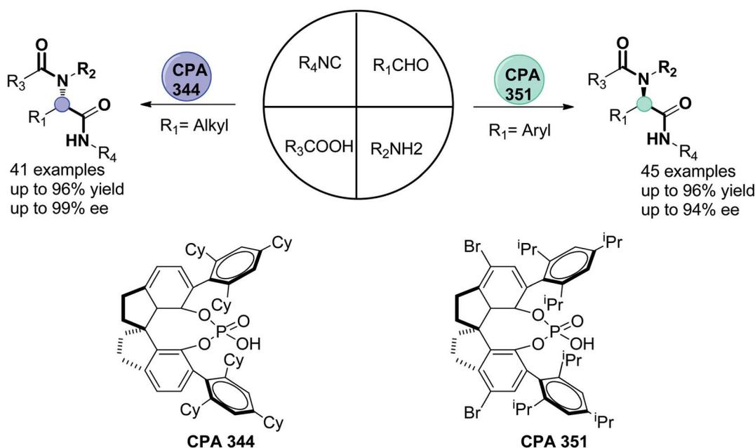
Fig. 6 Stereochemistry control of enantioselective four-component Ugi reaction.
