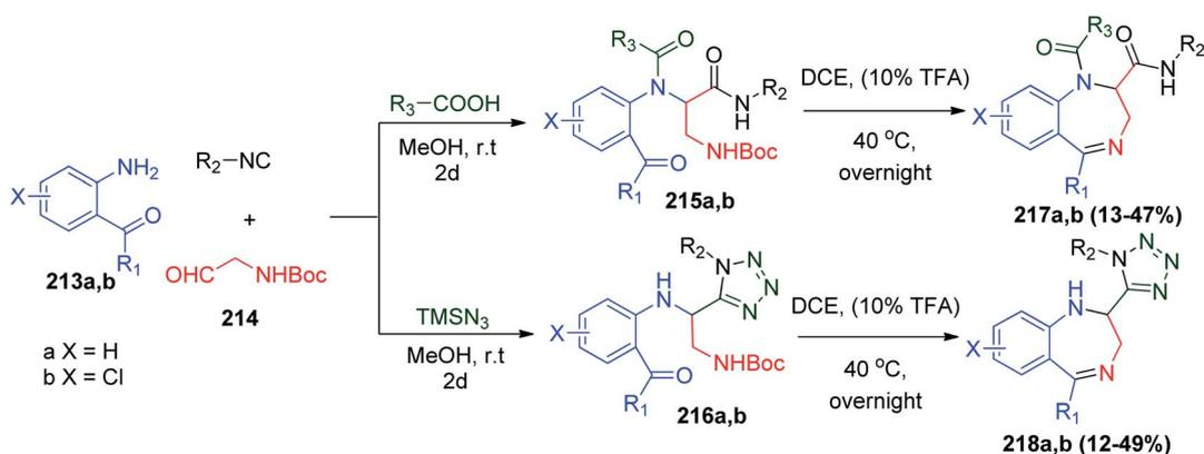
Scheme 45 Synthesis of 1,4-benzodiazepines derivatives **217a** and **218b** using Boc-glycinal **214**.
