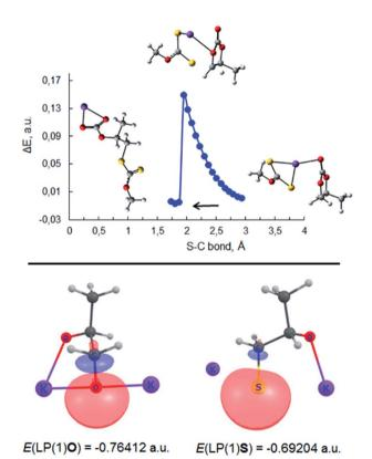
Fig. 7 Top: scan of total energy along the reaction coordinate for the attack of S $^-$  of PMX on the methylene carbon atom of PC (S $^-$ C bond formation) calculated at the m06-2x/6-311++G(d,p)/PCM level of theory (sulfur  $^-$  yellow, potassium  $^-$  purple, oxygen  $^-$  red). Bottom: images and energies of donor NBO of C1 oxygen of potassium propane-1,2-bis(olate) (3, Scheme 2) and sulfur atom of potassium 1-sulfidopropan-2-olate (III, Scheme 3) calculated at the same level of theory.
