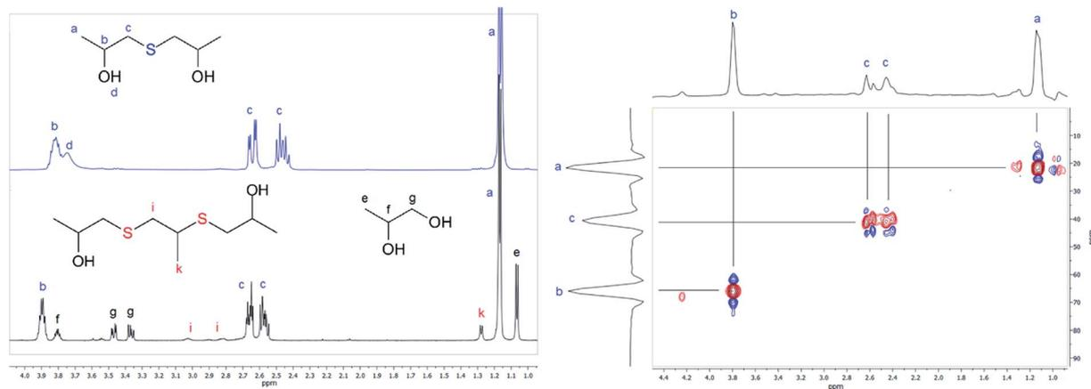
Fig. 3 Left:  $^1\text{H}$  NMR spectra of 1,1'-thiobis(propan-2-ol) (blue) dissolved in  $\text{CDCl}_3$  and powdered precipitate depicted in Fig. 2 dissolved in  $\text{D}_2\text{O}$ . Right: HSQC correlation spectra for the sulfide 1,1'-thiobis(propan-2-ol) dissolved in  $\text{CDCl}_3$ . Spectra were recorded at 25 °C.
