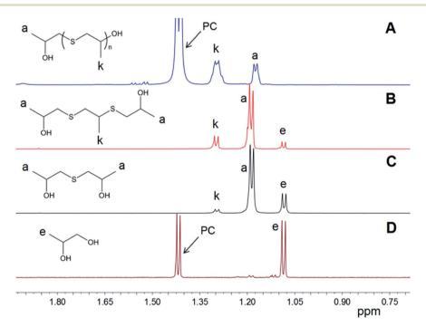
Fig. 5 Fragments of  $^1H$  NMR spectra in the region of methyl protons for polypropylene sulfide in CDCl<sub>3</sub> (A); precipitates obtained in the course of the reaction between PC and PMX in bulk at 100  $^{\circ}$ C (B) and 80  $^{\circ}$ C (C) and the precipitate formed in the course of the reaction between PC and PMX at 90  $^{\circ}$ C in the presence of water (10%). Spectra (B–D) were recorded in D<sub>2</sub>O at 25  $^{\circ}$ C.
