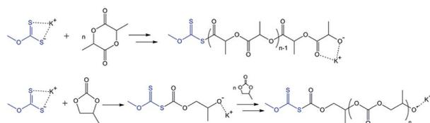
Scheme 1 Top: previously described lactide polymerization initiated by xanthate-functionalized initiators<sup>26</sup> and the proposed route for the polymerization of PC in the presence of potassium methylxanthate based on the same idea (bottom).
