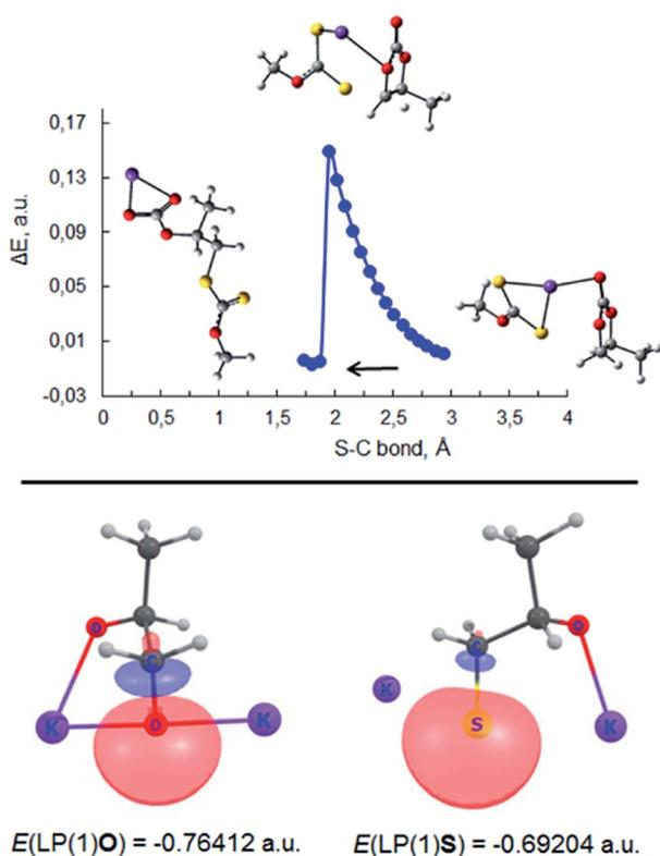
Fig. 7 Top: scan of total energy along the reaction coordinate for the attack of  $S^-$  of PMX on the methylene carbon atom of PC (S–C bond formation) calculated at the m06-2x/6-311++G(d,p)/PCM level of theory (sulfur – yellow, potassium – purple, oxygen – red). Bottom: images and energies of donor NBO of C1 oxygen of potassium propane-1,2-bis(olate) (3, Scheme 2) and sulfur atom of potassium 1-sulfidopropan-2-olate (III, Scheme 3) calculated at the same level of theory.
