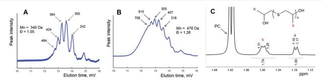
Fig. 4 GPC traces of oligomers synthesized in the course of the reaction between EC (A) and PC (B) with PMX carried out in bulk at 100 °C and a fragment of the <sup>1</sup>H NMR spectrum (right) of polypropylene sulfide-based oligomers recorded in CDCl<sub>3</sub> at 25 °C.
