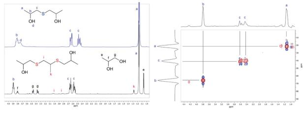
Fig. 3 Left:  $^{1}$ H NMR spectra of 1,1'-thiobis(propan-2-ol) (blue) dissolved in CDCl<sub>3</sub> and powdered precipitate depicted in Fig. 2 dissolved in D<sub>2</sub>O. Right: HSQC correlation spectra for the sulfide 1,1'-thiobis(propan-2-ol) dissolved in CDCl<sub>3</sub>. Spectra were recorded at 25  $^{\circ}$ C.
