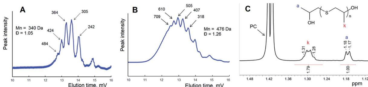
Fig. 4 GPC traces of oligomers synthesized in the course of the reaction between EC (A) and PC (B) with PMX carried out in bulk at 100 °C and a fragment of the  $^1\text{H}$  NMR spectrum (right) of polypropylene sulfide-based oligomers recorded in  $\text{CDCl}_3$  at 25 °C.
