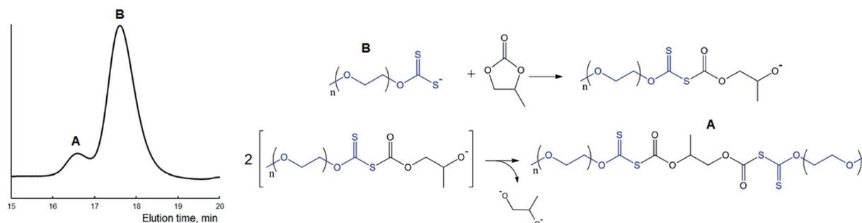
**Fig. 6** GPC trace of polymer (A) obtained in the course of the reaction between  $MPEG_{2k}X$  (B) and PC at  $100\text{ }^{\circ}C$  in bulk and a scheme displaying the proposed reactions (see also Scheme 2A). Potassium ions are omitted for clarity.
