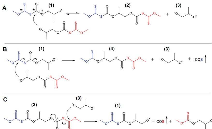
**Scheme 2** (A and B) Interactions of two thiocarbonates (growing chains, **1**) via chain termination reactions with the subsequent formation of neutral species (**2** and **4**) and alkoxide **3**. (C) Attack of alkoxide propane-1,2-bis(olate) on the C=S carbon of the xanthate group of **2** accompanied by COS release and formation of initial thiocarbonate **1** and intermediate 1-((methoxycarbonothioyl)thio)propan-2-olate. Potassium ions are omitted for clarity.
