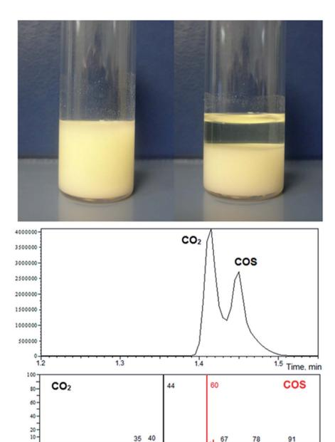
Fig. 2 Top: images of the slurry containing solid products and residual PC captured immediately after the completion of the reaction between PC and PIBX (PC/PIBX = 25/1) carried out at  $100 \,^{\circ}$ C (left) and after a few hours of relaxation. Bottom: GC traces for the gases evolved in the course of the reaction between PC and PIBX and mass-spectra of the identified substances.
