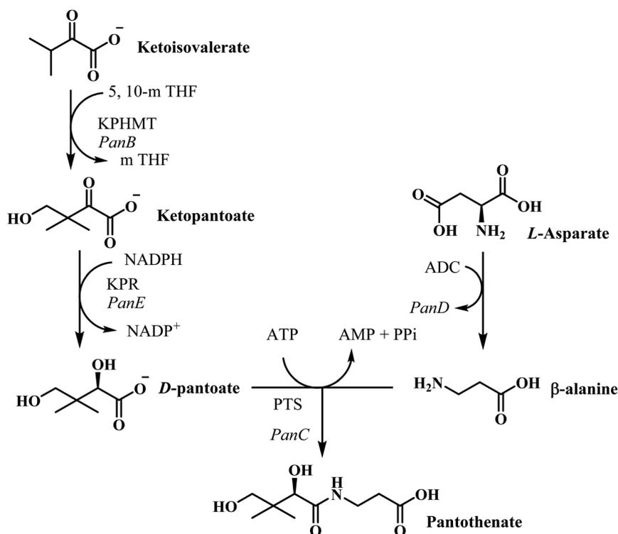
Fig. 2 Pantothenate biosynthesis pathway in *E. coli*.<sup>22</sup> The enzymes are KPHMT, ketopantoate hydroxymethyltransferase;<sup>20</sup> KPR, ketopantoate reductase; ADC, aspartate decarboxylase;<sup>23</sup> PS, pantothenate synthetase; 5,10-mTHF, 5,10-methylene tetrahydrofolate.
