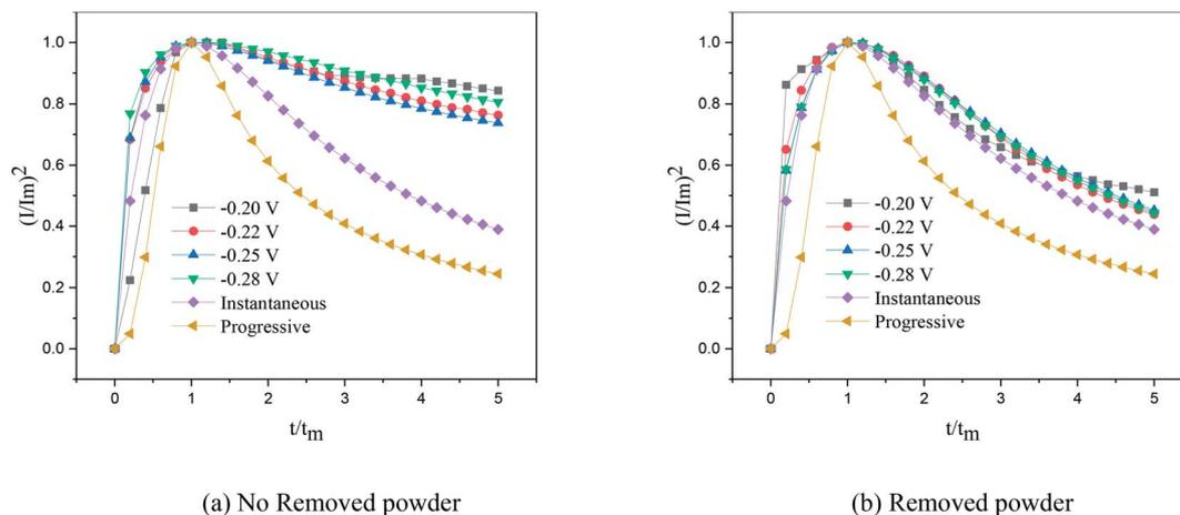
Fig. 7 Dimensionless curves of copper deposition on stainless steel electrodes.
