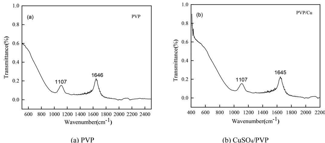
Fig. 11 Infrared spectra of the different electrolytes: (a) PVP (b) CuSO<sub>4</sub>/PVP.
