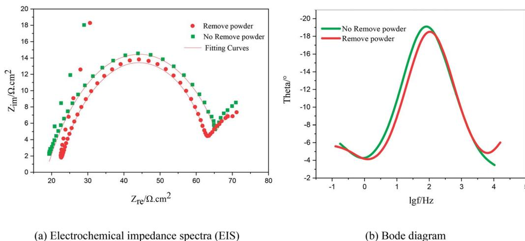
Fig. 9 Electrochemical impedance spectra and Bode diagram of copper under the same potential and different electrolytic conditions. (a) Impedance spectra; (b) Bode diagrams.
