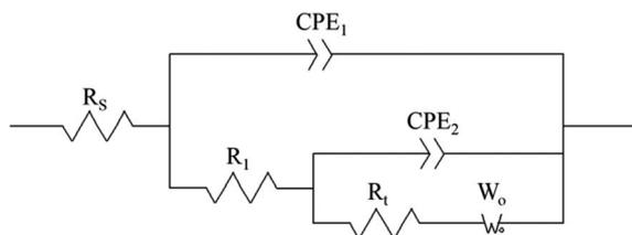
Fig. 10 Equivalent circuit diagram of 0.1 g L<sup>-1</sup> PVP electrolyte at the same potential and different electrolytic conditions.  $R_s$  is the solution resistance,  $R_1$  is the membrane resistance,  $CPE_2$  is the interface capacitance of the PVP membrane,  $R_t$  is the transfer resistance,  $CPE_1$  is the double-layer capacitance, and  $W_o$  is the diffusion process.
