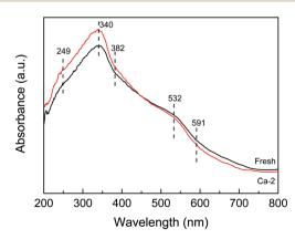
Fig. 3 XRD patterns of the fresh and different Ca-poisoned catalysts. Fig. 5 UV-vis DRS spectra of the fresh and the Ca-2 catalysts.
