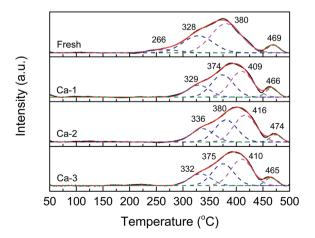
Fig. 7  $\,\mathrm{H_{2}\text{-}TPR}$  profiles of the fresh and different Ca-poisoned catalysts.
