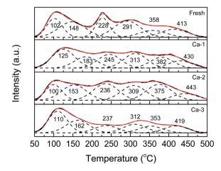
Fig. 8  $\,\mathrm{NH_{3}}\text{-}\mathrm{TPD}$  profiles of the fresh and different Ca poisoned catalysts.
