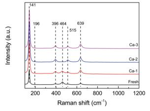
Raman spectra of the fresh and different Ca poisoned catalysts.
