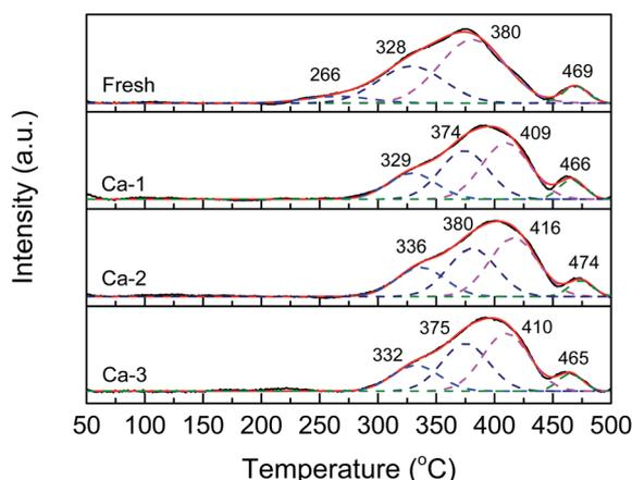
Fig. 7  $\text{H}_2$ -TPR profiles of the fresh and different Ca-poisoned catalysts.
