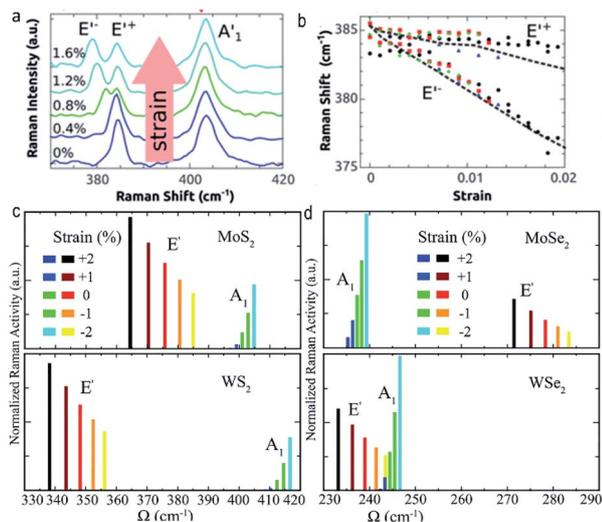
Fig. 2 (a) Raman spectra of monolayer MoS<sub>2</sub> under different strain. (b) Strain-dependent Raman frequency of mode E' in monolayer MoS<sub>2</sub>. Reproduced with permission.<sup>50</sup> Copyright 2013, American Chemical Society. The calculated strain responses of Raman activities of monolayer (c) MoS<sub>2</sub> and WS<sub>2</sub> and (d) MoSe<sub>2</sub> and WSe<sub>2</sub>. Reproduced with permission.<sup>53</sup> Copyright 2018, American Physical Society.
