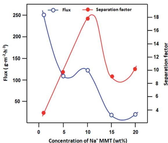
Fig. 10 Variation in the pervaporation flux and separation factor versus the concentration of Na<sup>+</sup>MMT for the separation of azeotropic composition of the ethanol–water mixture at 30 °C.
