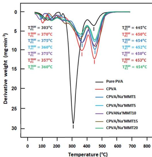
Fig. 6 DTG thermograms of pure PVA, CPVA and CPVA/Na<sup>+</sup>MMT nanocomposites containing different Na<sup>+</sup>MMT contents.
