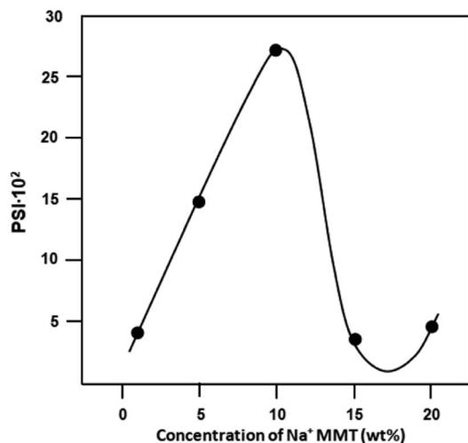
Fig. 12 Variation in PSI versus the concentration of Na<sup>+</sup>MMT for the separation of azeotropic composition of ethanol–water mixture at 30 °C.
