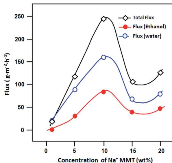
Fig. 11 Variation in component fluxes versus the concentration of Na<sup>+</sup>MMT for the separation of azeotropic composition of the ethanol–water mixture at 30 °C.
