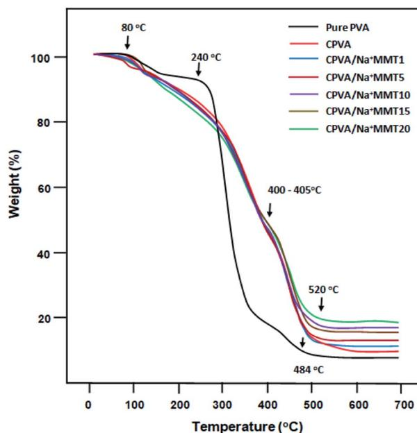
Fig. 5 TGA thermograms of pure PVA, CPVA and CPVA/Na<sup>+</sup>MMT nanocomposites containing different Na<sup>+</sup>MMT contents.
