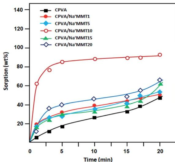
Fig. 9 Plots of the variation of swelling of the nanocomposite membranes in an azeotropic composition 4 : 96 water/ethanol mixture at room temperature as a function of time.
