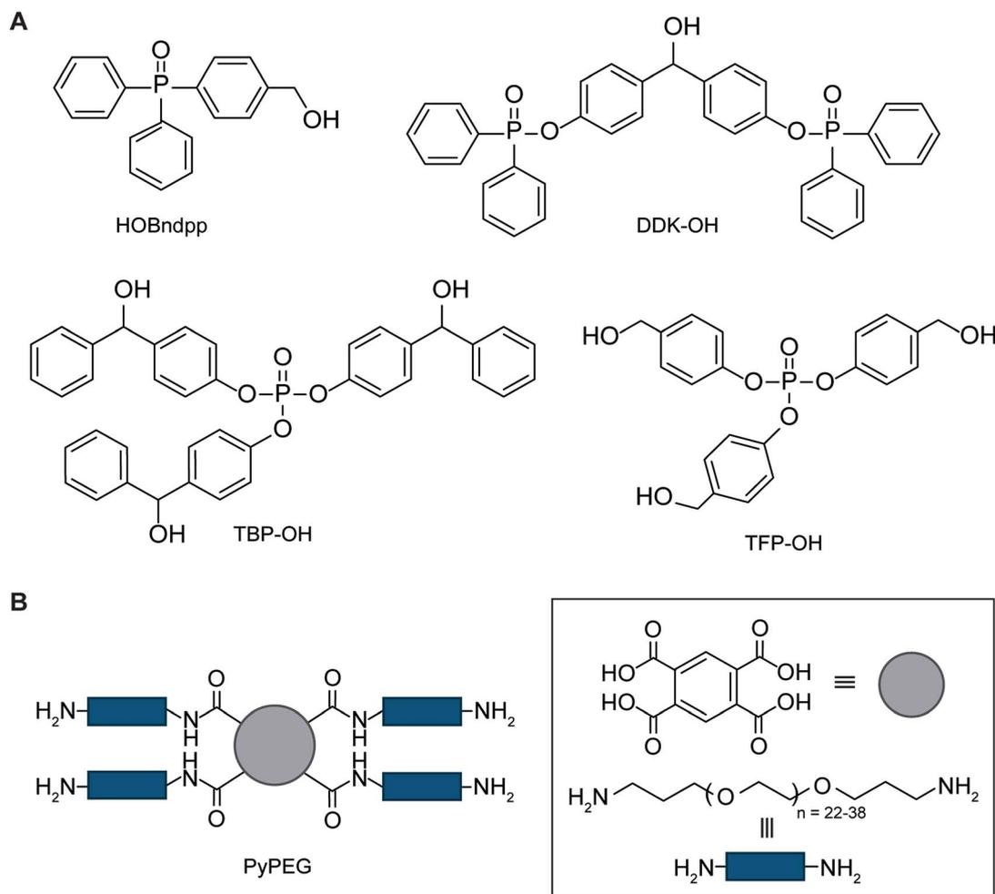
Fig. 10 Chemical structures of (A) Benzyl alcohol anchors for LPPS with group-assisted purification based on diphenylphosphine oxide (Bndpp),<sup>113</sup> tri(4-formylphenyl) phosphonate (TFP),<sup>114</sup> tri(4-benzoylphenyl) phosphate (TBP),<sup>115</sup> and diphenylphosphinyloxy diphenyl ketone (DDK)<sup>116</sup> scaffolds, and (B) branched 6.2 kDa PEG-based anchor PyPEG for membrane-enhanced peptide synthesis (MEPS).<sup>120</sup>
