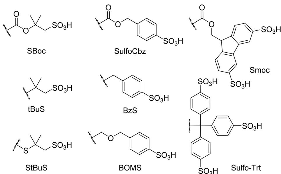
Fig. 6 Sulfonate-derived protecting groups developed by Kolmar and co-workers and commercialised by the company Sulfotools.<sup>95,96</sup>
