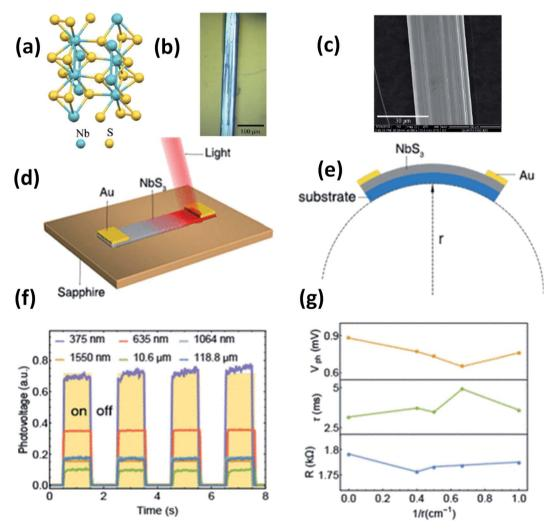
Fig. 15 (a) The crystal structure of NbS<sub>3</sub>. (b) Optical microscopy and (c) SEM images of a NbS<sub>3</sub> crystal. Schematic diagrams of (d) a NbS<sub>3</sub> photodetector and (e) bending conditions. (f) ON–OFF photovoltage curves at room temperature and (g) resistance, response time, and photovoltage data under different bending conditions. Reprinted with permission from ref. 151, copyright: 2020, American Chemical Society.
