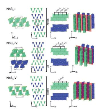
Fig. 5 The crystal structure of  $NbS_{3-IV}$ ,  $NbS_{3-IV}$ , and  $NbS_{3-V}$ : unit cells, chain cross-sections, layers, and perspective views. Reproduced with permission from ref. 55, copyright: 2017, Application Infrastructure Provider.
