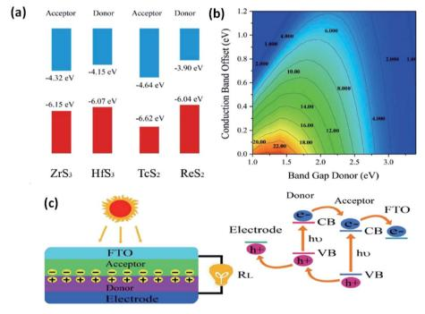
Fig. 13 The application of  $MX_3$  heterostructures to solar cells. (a) Band offsets of  $ZrS_3/HfS_3$  and  $TcS_2/ReS_2$  with the vacuum level as zero reference. (b) PCE contours obtained as a function of the donor band gap and conduction band offset. (c) A schematic illustration of thin-film solar cells with the associated mechanism. Republished with permission from ref. 33, permission conveyed through Copyright Clearance Center, Inc.
