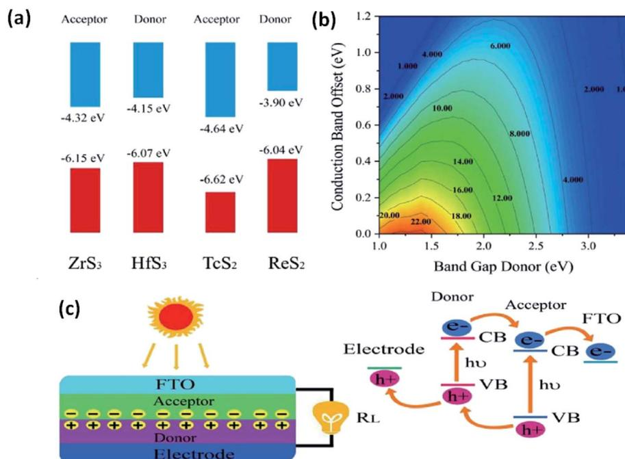
Fig. 13 The application of MX<sub>3</sub> heterostructures to solar cells. (a) Band offsets of ZrS<sub>3</sub>/HfS<sub>3</sub> and TcS<sub>2</sub>/ReS<sub>2</sub> with the vacuum level as zero reference. (b) PCE contours obtained as a function of the donor band gap and conduction band offset. (c) A schematic illustration of thin-film solar cells with the associated mechanism. Republished with permission from ref. 33, permission conveyed through Copyright Clearance Center, Inc.
