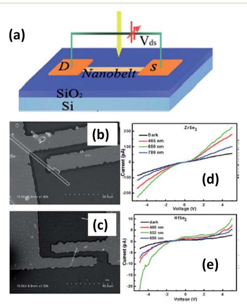
Fig. 14 (a) A schematic illustration of a ZrSe<sub>3</sub> and HfSe<sub>3</sub> single nanobelt photodetector. SEM images of (b) ZrSe<sub>3</sub> and (c) the HfSe<sub>3</sub> photodetector. I-V characteristics of (d) ZrSe<sub>3</sub> and (e) the HfSe<sub>3</sub> nanobelt photodetector. Republished with permission from ref. 129, permission conveyed through Copyright Clearance Center, Inc.
