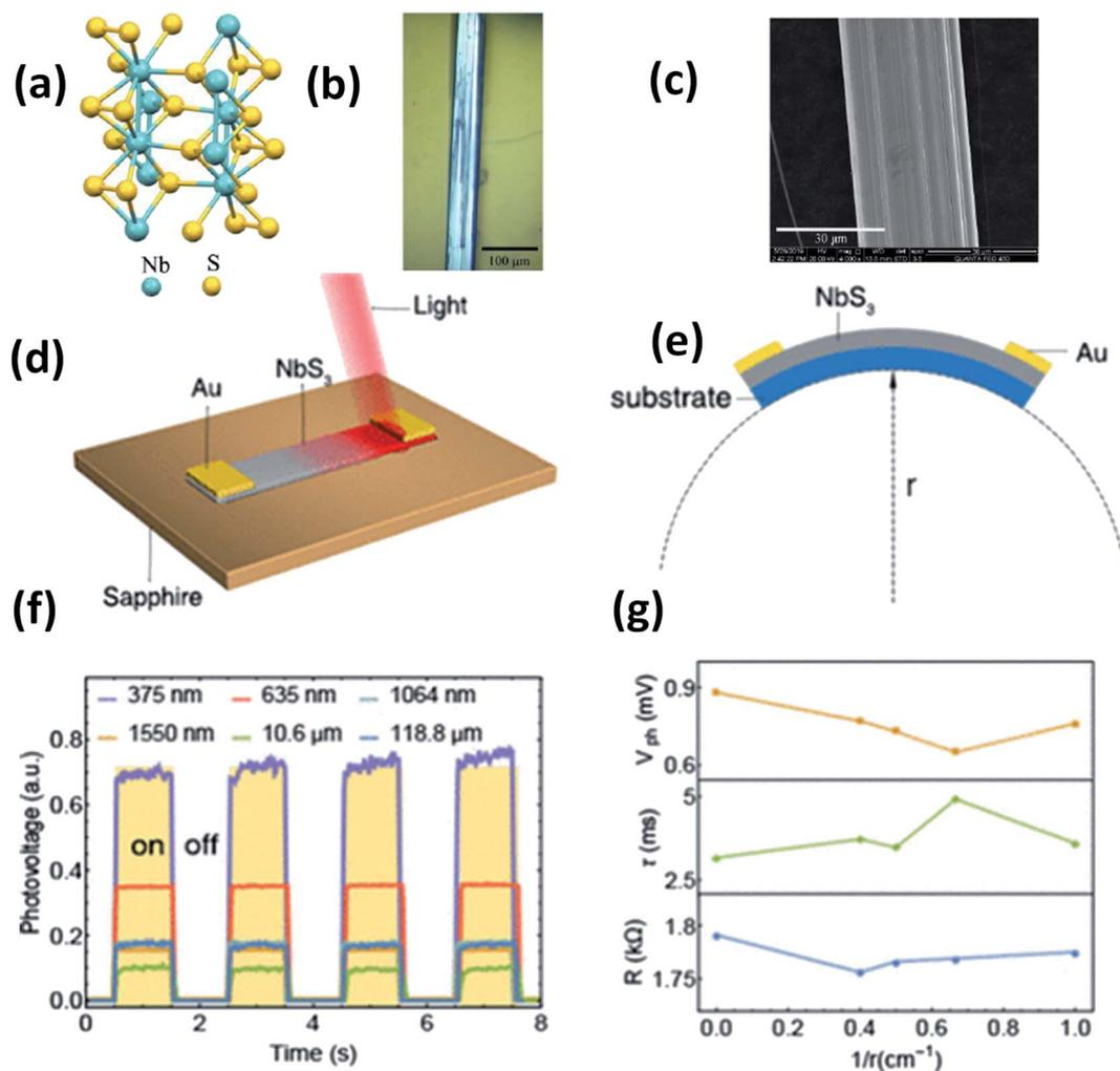
Fig. 15 (a) The crystal structure of  $\text{NbS}_3$ . (b) Optical microscopy and (c) SEM images of a  $\text{NbS}_3$  crystal. Schematic diagrams of (d) a  $\text{NbS}_3$  photodetector and (e) bending conditions. (f) ON–OFF photovoltage curves at room temperature and (g) resistance, response time, and photovoltage data under different bending conditions. Reprinted with permission from ref. 151, copyright: 2020, American Chemical Society.
