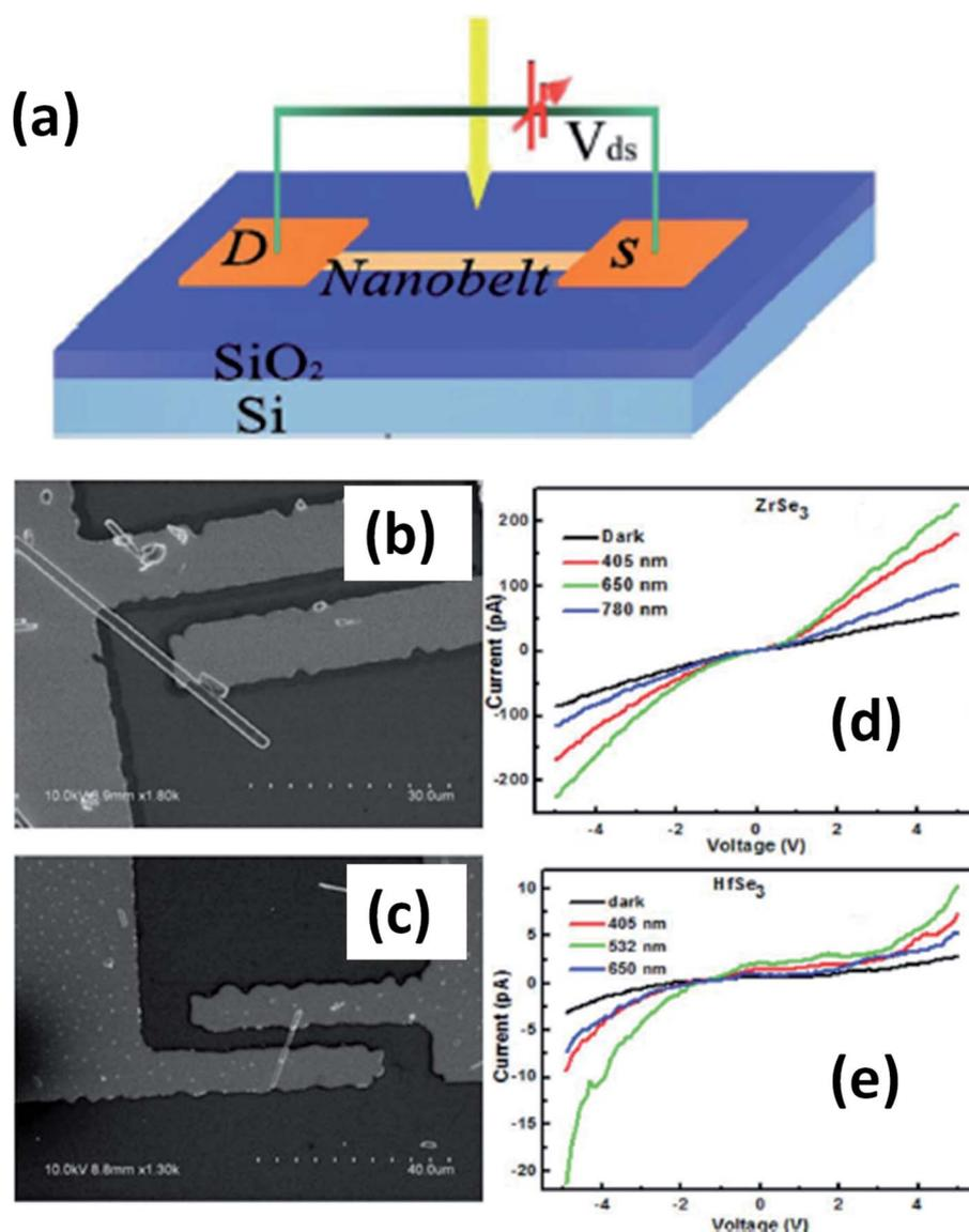
Fig. 14 (a) A schematic illustration of a  $\text{ZrSe}_3$  and  $\text{HfSe}_3$  single nanobelt photodetector. SEM images of (b)  $\text{ZrSe}_3$  and (c) the  $\text{HfSe}_3$  photodetector.  $I$ - $V$  characteristics of (d)  $\text{ZrSe}_3$  and (e) the  $\text{HfSe}_3$  nanobelt photodetector. Republished with permission from ref. 129, permission conveyed through Copyright Clearance Center, Inc.
