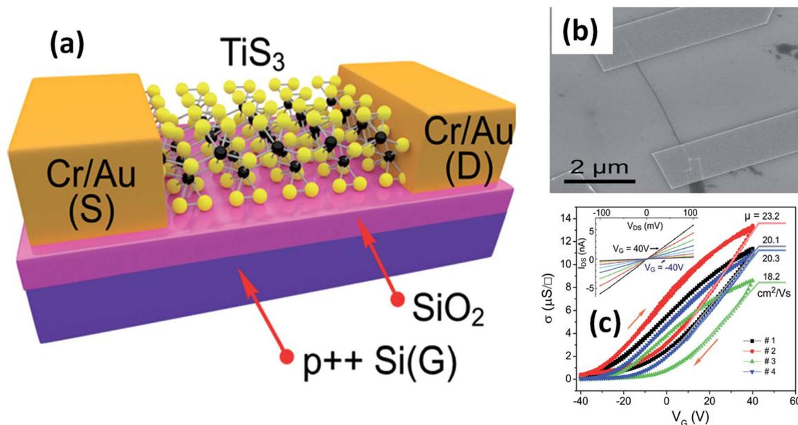
Fig. 11 Few-layered  $\text{TiS}_3$  FETs. (a) A schematic diagram and (b) an SEM image of a typical FET. (c) Conductivity vs. gate voltage dependencies of four different fabricated FETs, with the inset showing drain source current vs. drain source voltage at different gate voltages. Reproduced with permission from ref. 124, copyright: 2015, Royal Society of Chemistry.
