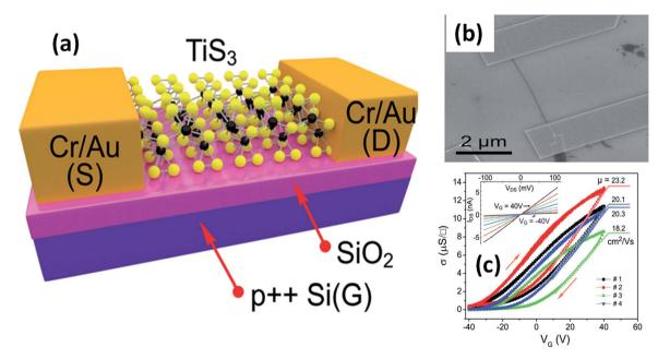
Fig. 11 Few-layered TiS<sub>3</sub> FETs. (a) A schematic diagram and (b) an SEM image of a typical FET. (c) Conductivity vs. gate voltage dependencies of four different fabricated FETs, with the inset showing drain source current vs. drain source voltage at different gate voltages. Reproduced with permission from ref. 124, copyright: 2015, Royal Society of Chemistry.
